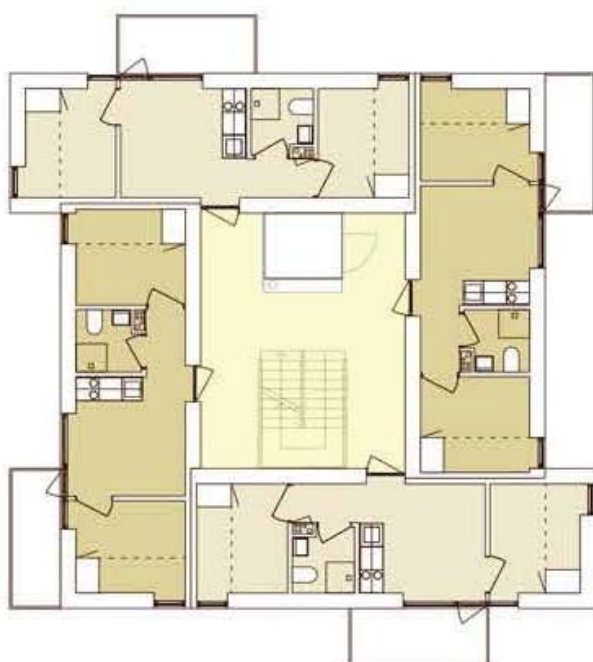
Figure 13 A floor with four apartments (33 m 2 ) of two rooms, kitchen and bathroom in Venligbolig Plus. Source: ONV Architects, 2019.
