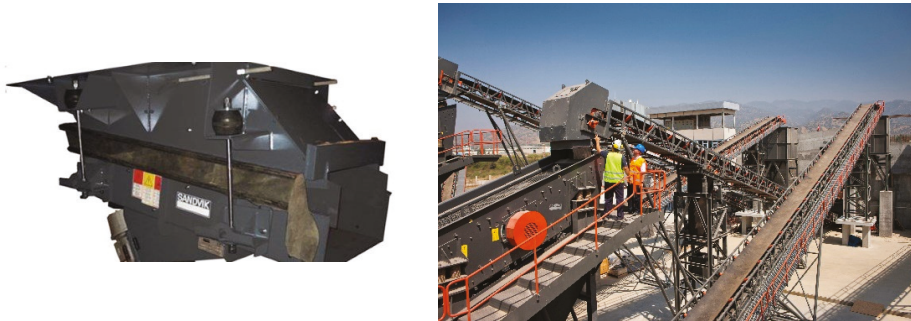
Figure 1.7 Vibrating feeder with dust encapsulation (left), and conveyors (right).
