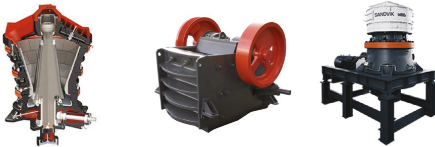
Figure 1.9 Different types of compression crushers, gyrotory, jaw, and cone [4].
