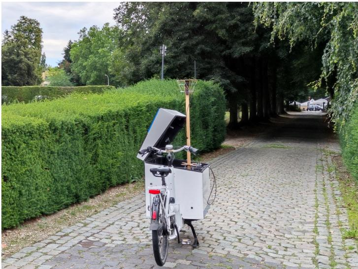
**Figure 2:** Transmit node with a single dipole antenna.
