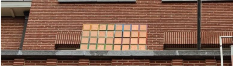
(b)  $4 \times 8$  URA**Figure 1:** Antenna array configurations.
