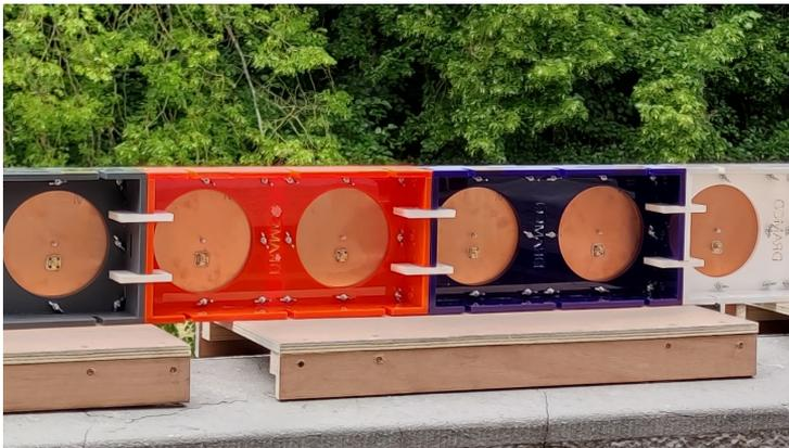
**Figure 3:** Multiple modular antenna holders connected.
