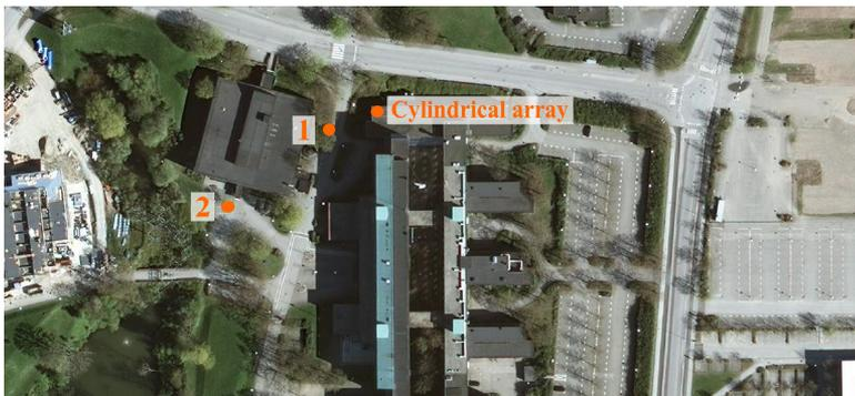
**Figure 2:** The outdoor scenario for both LOS (position 1) and NLOS (position 2). The base station has a cylindrical array and is positioned on the roof. The users were moving within a circle with a diameter of 5 m.
