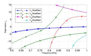
Fig. 1. Characteristic eigenvalues of a 130 mm  $\times$  66 mm chassis with and without shorted metal strips along the longer ends.
