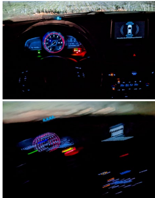
Figure 2: Illustration of phantom arrays. Photo: J.Ledig
