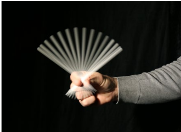
Figure 2: Illustration of stroboscopic effect. Photo: J.Rydeman
