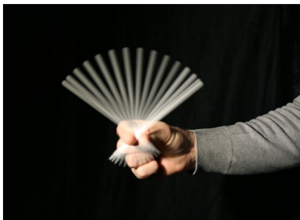
Figure 2: Illustration of stroboscopic effect. Photo: J.Rydeman
