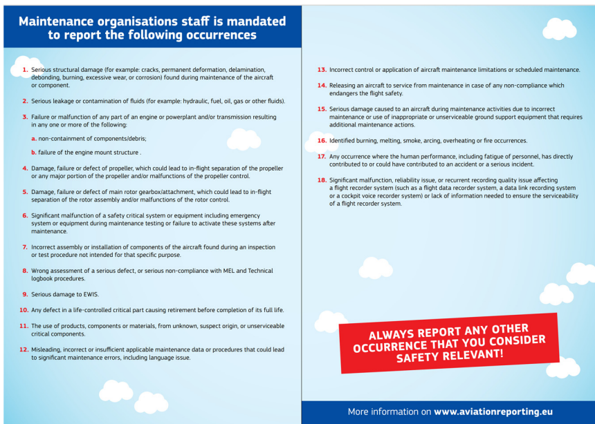
Figure 10b. Safety reporting information leaflet for maintenance personnel (inside cover) (ECCAIRS 2020).
