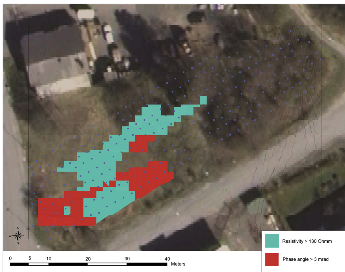
Fig. 8. Map showing the highest resistivity- and phase values in the sandy till ( -4 to -14 mamsl), obtained through interpolation of the resistivity and phase values in the CPA inverted 2D sections.
