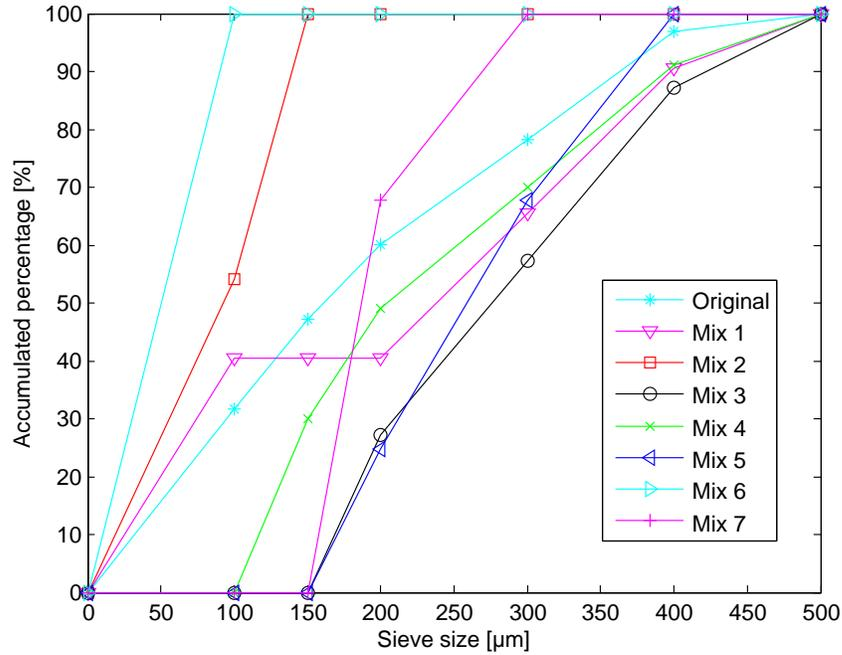
Figure 19: Particle size distribution for different mixing relationships.
