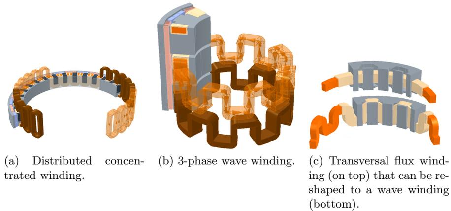
Figure 34: Different coil designs used for motor prototypes.
