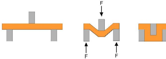
Figure 37: Principle of winding forming process, illustrated as 3 interacting dies (grey) forming part of a winding (orange) [55].
