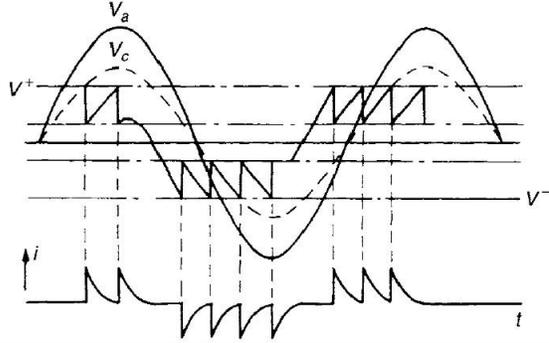
Figure 11: Sequence of cavity breakdown under alternating voltages [12].
