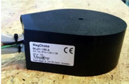
Figure 57: MagChoke, 50  $\mu\text{H}$ , 150 A, 118 mm diameter, 52 mm height.
