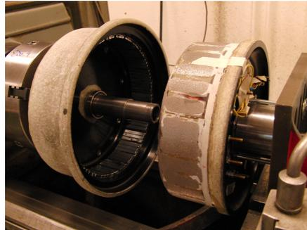
Figure 52: Mounting of stator 1 in to the rotor.
