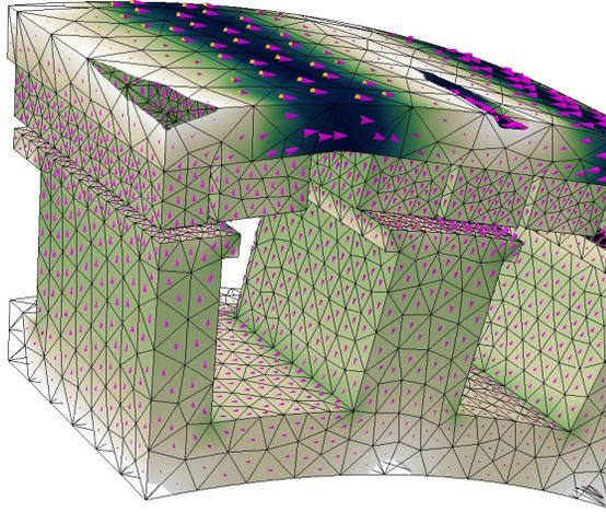
Figure 4: Flux linkage simulation for SM<sup>2</sup>C stator core. [9]
