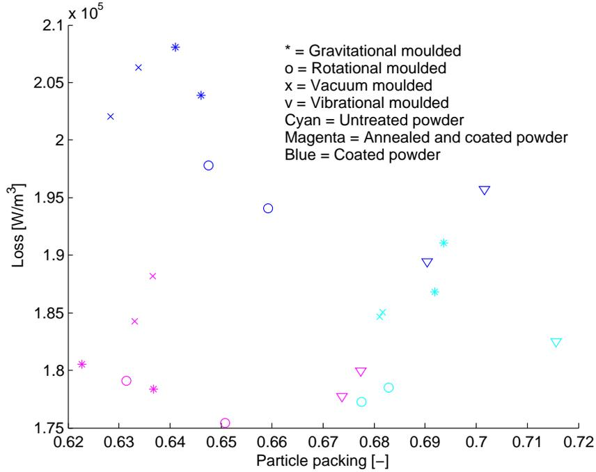
Figure 26: Comparison of SM<sup>2</sup>C loss at 10 kHz and 0.1 T, with different powder treatments and moulding processes.
