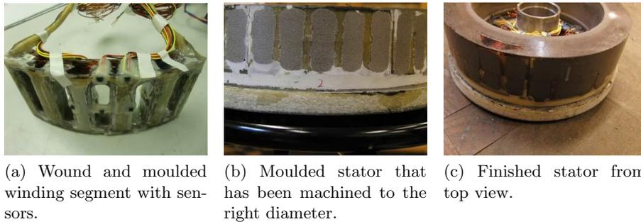
Figure 28: Production phases for SM<sup>2</sup>C moulded stator, Stator number one [46].
