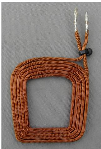
Figure 42: Uncoated coil [11].
