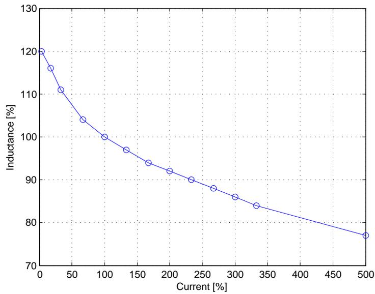
Figure 59: Inductance versus current on a MagChoke. L nominal = 100 % and I nominal = 100 %.
