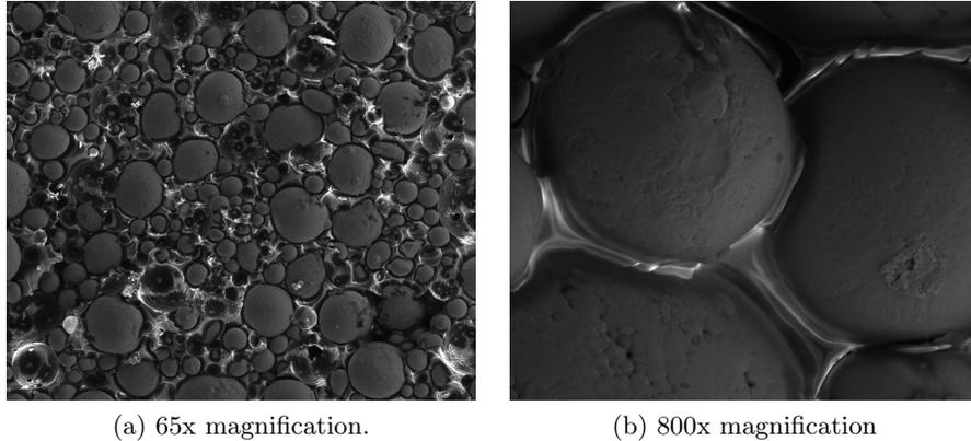
Figure 21: SEM picture of a fractured SM<sup>2</sup>C surface [18].
