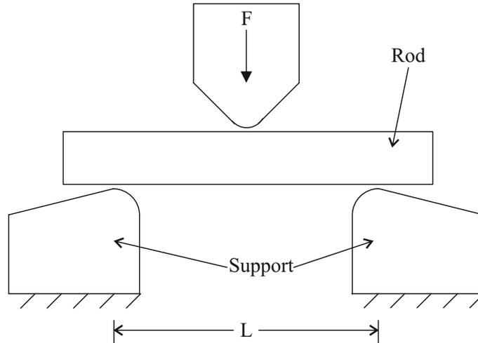
Figure 17: Schematic figure over the three point bend fixture.
