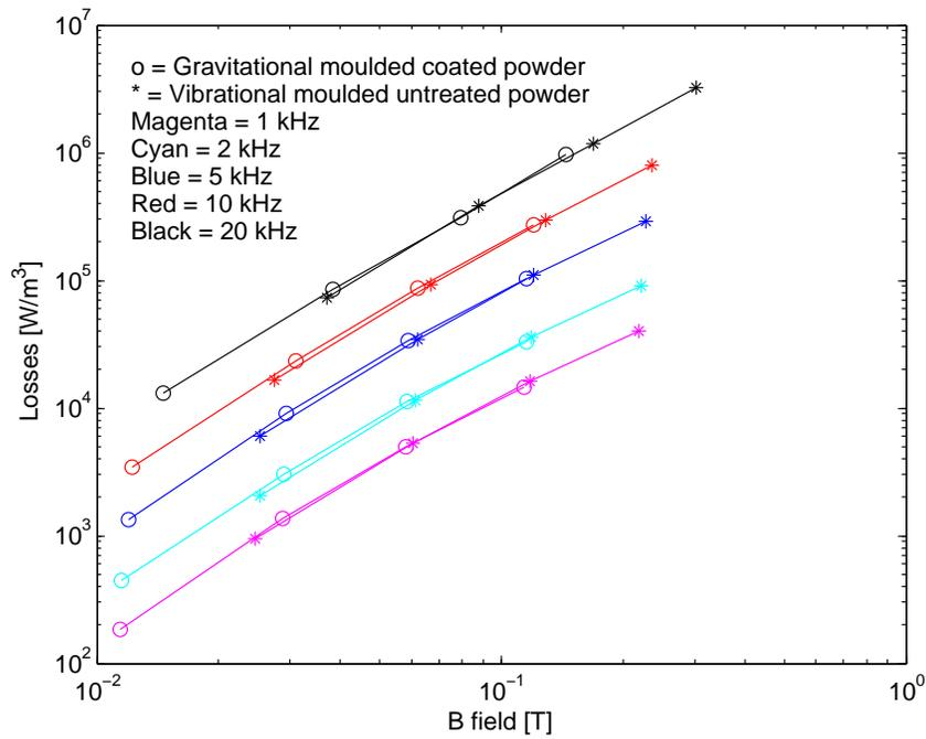
Figure 33: Loss as a function of B field at different frequencies for a vibrational moulded sample using untreated powder and a gravitational moulded sample with coated powder.
