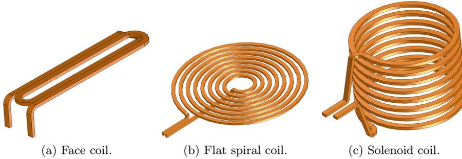
Figure 2: Induction heater coil configurations.
