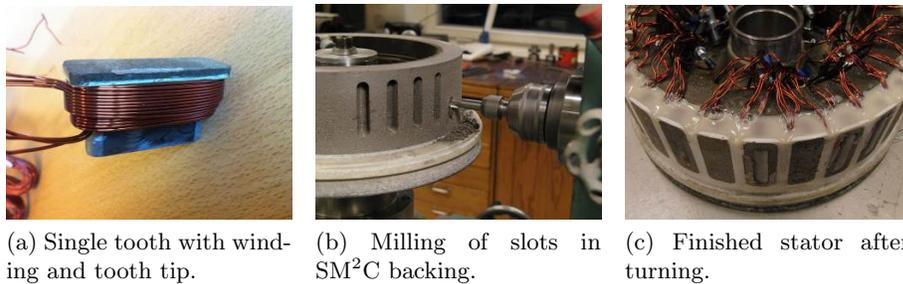
Figure 29: Production phases of single SMC tooth wound stator with SM<sup>2</sup>C moulded backing, Stator number two [46].
