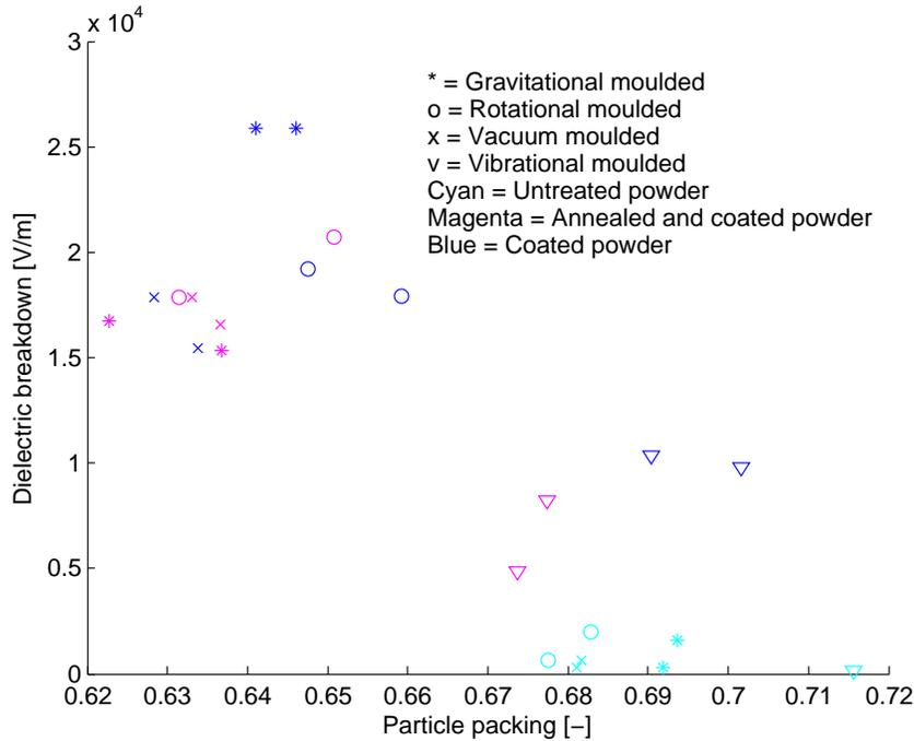
Figure 27: Dielectric breakdown comparison of different samples.
