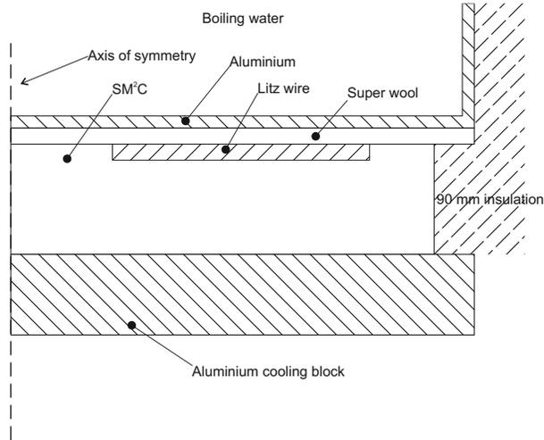
Figure 48: Schematic of test setup 2 with aluminium load [32].
