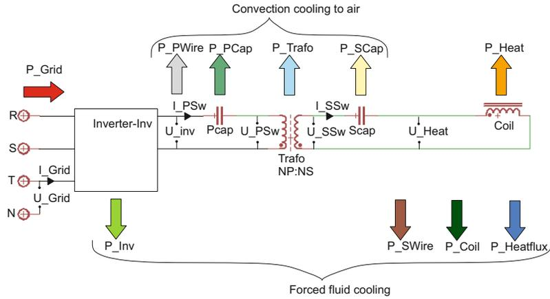
Figure 3: Schematic and loss chart over an induction circuit, including workpiece.
