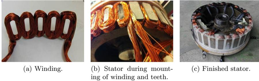
Figure 30: Production phases of SMC tooth wound stator with SM<sup>2</sup>C moulded backing, Stator number three [46].
