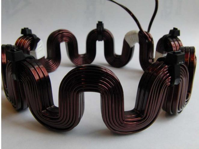
Figure 36: Wave winding with 35 mm press height [55].
