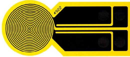
Figure 16: Kapton sensor used for measurements [32].
