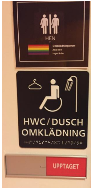
Figure 1: The sign shows two types of users for this changing room: wheelchair users and people of all gender/or no gender. Instead it should show the function of the room – an individual changing room.
