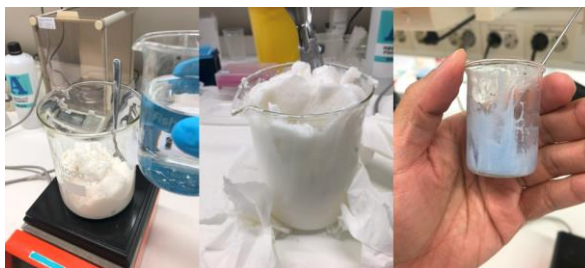
Figure 11a. Step 1) Cream base preparation: mix glyceryl stearate SE and water (final concentration: 15% glyceryl stearate w/w) & test for equal distribution of additional substance by mixing the cream with textile dye mix test preparation in petrolatum to observe whether the color can be blended.
