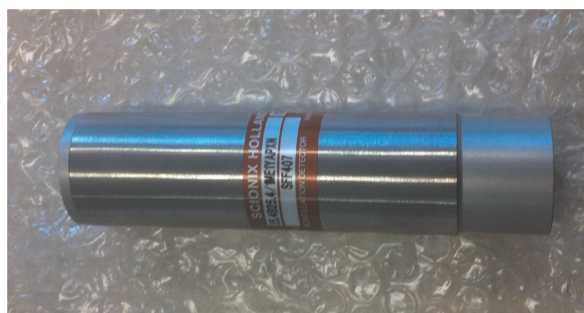
Fig. 2. Photograph of a YAP detector. A 1 in (diameter) \times 1 in (height) crystal has been mounted on a 1 in (diameter) \times 10 cm (length) PMT.
