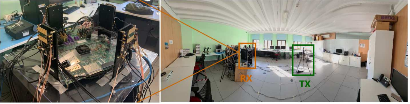
Fig. 1: Left : The 4 RX antenna arrays connected to the SIVERS FPGA to perform real-time processing. Right : Room at IMDEA with TX and RX placed at positions \mathbf{p}_1 = [0 \text{ m}, 2.4 \text{ m}] and \mathbf{p}_{\text{RX}} = [0, 0] , respectively.
