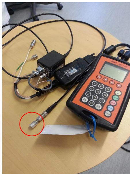
Figure1. The 4 mm 2 Si diode, indicated by a circle, connected to a charge-sensitive preamplifier (2003BT) and a digital portable multichannel analyzer (DigiDart™).
