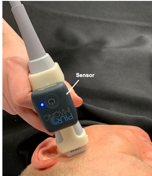
Figure 13. The sensor clips onto a standard ultrasound transducer, and conveys the transducer's position in time and space to a workstation via Bluetooth. The examination requires only a single sweep over the target tissue, and the data are stored for further analysis.
