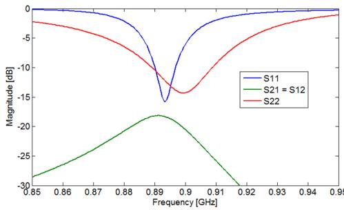
Fig. 4. Scattering parameters of the two-port antennas.
