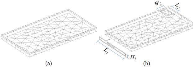
Fig. 3. (a) Initial bezel-loaded chassis, (b) Final design with feed elements embedded into chassis ( $L_1 = 60$  mm  $H_1 = 5$  mm,  $L_2 = 16.4$  mm  $W_2 = 11.4$  mm).
