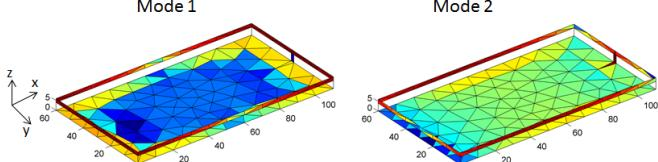
Figure 1: Characteristic currents of Modes 1 and 2 at 0.89 GHz.
