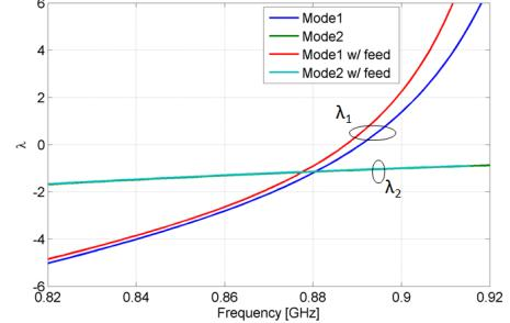
Fig. 5. Eigenvalues of both modes with and without the feeding structures.
