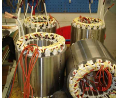
Fig. 6.4 Illustration of the VCE electrical machine stators
