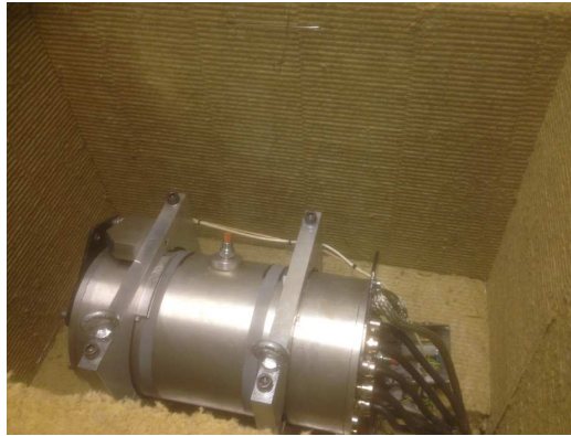
Fig. 6.13 EM3 placed inside a temperature insulated chamber [107]
