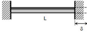
Fig. 4.1 Bar with both ends fixed [75]
