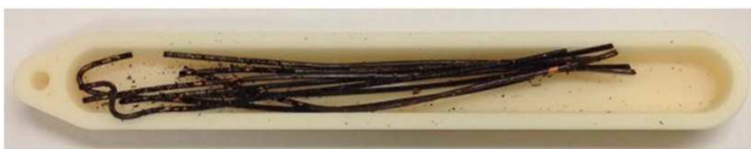
Fig. 7.1 Picture of the enameled wires after thermal stress of 275°C for 168 hours seated in the alumina boat crucible
