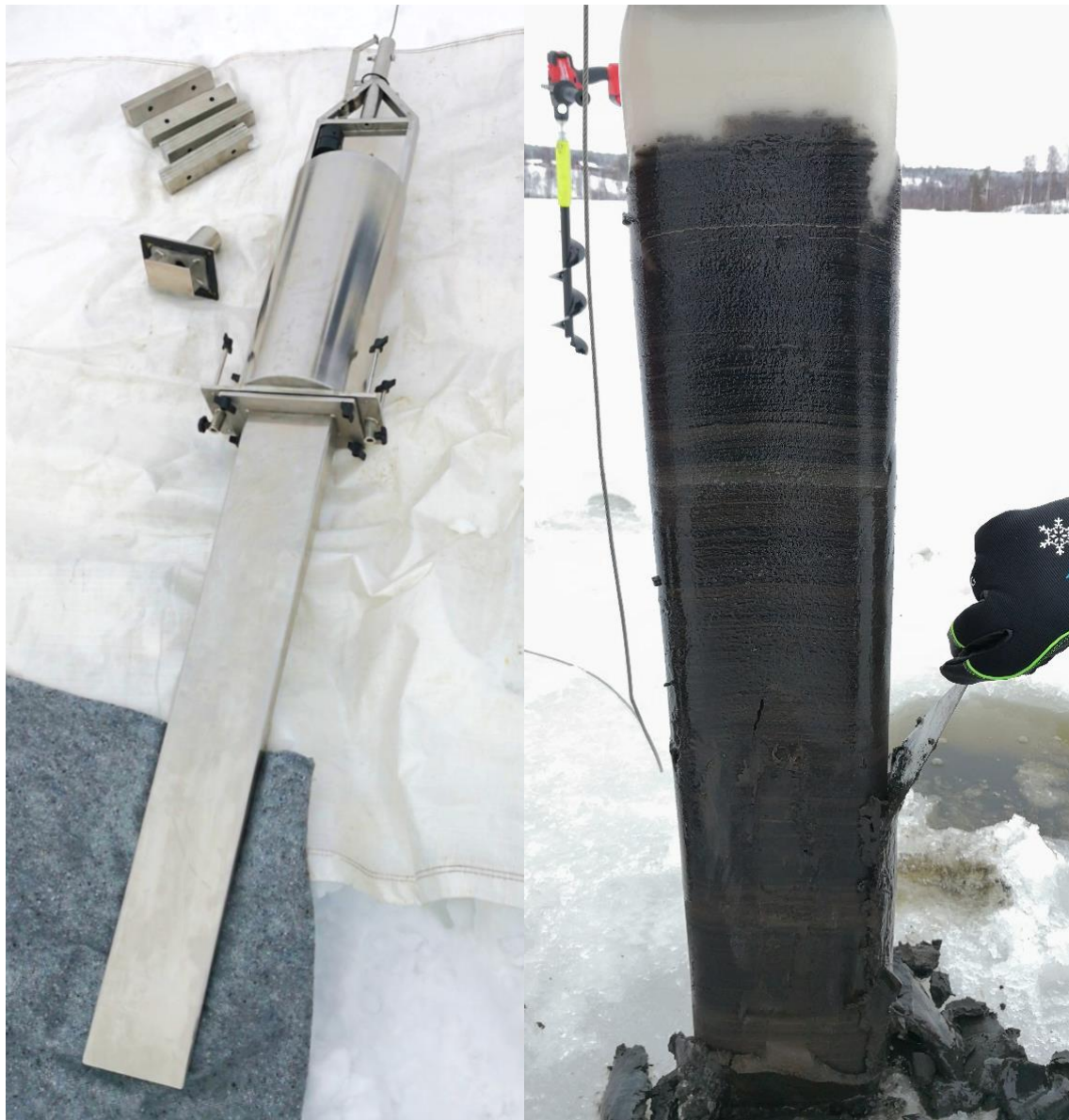
Figure 17. The freeze corer (Renberg and Hansson, 2010) used for sampling (left) and the freshly retrieved sediment sequence from Kassjön in March 2019 (left).
