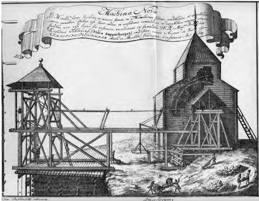
Figure 2. Polhem's hoisting machine at the mine "Blankstöten," Falun, Sweden. Published in Swedenborg's Dædalus Hyperboreus II (1716), and later on also in his De cupro (1734.)
