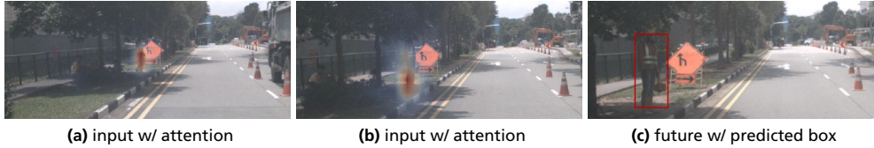
Figure 3.1: Emergent tracking capabilities visualized through attention maps, showing how the model learns to associate objects across frames without explicit tracking supervision. Illustration from Paper 1.
