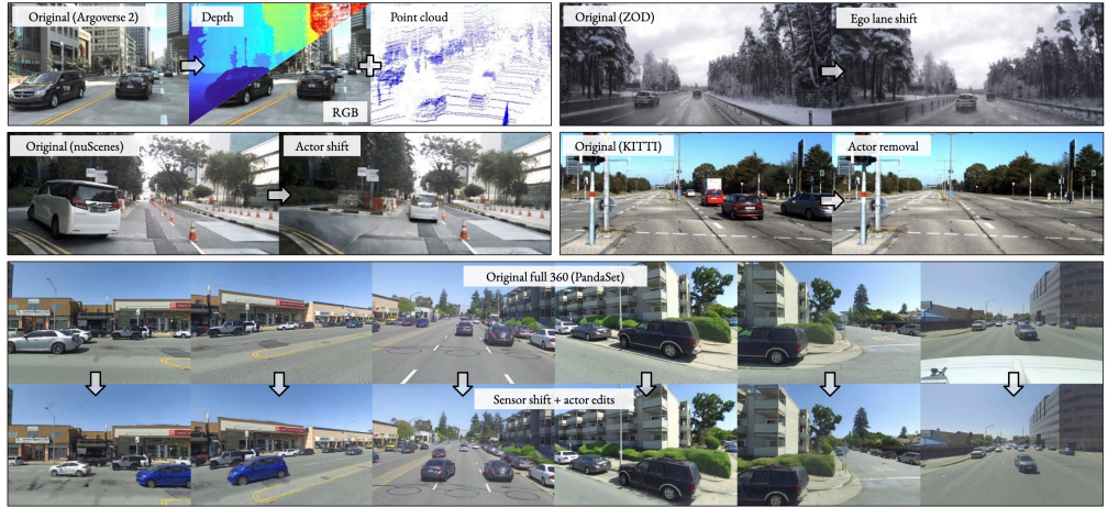
Figure 4.4: Qualitative examples showcasing the capabilities of NeuRAD. At the core is the ability to accurately re-render images, depth maps, and point clouds. By manipulating pose of the view that is rendered one can simulate a novel driving trajectory (shown on ZOD) and/or a different mounting position of the sensor (shown on PandaSet). Furthermore, since NeuRAD uses an explicit decomposition of static scene and dynamic actors, the actors can be removed or modified (shown on KITTI, NuScenes). All capabilities can of course be combined, resulting in realistic surround-consistent novel scenario simulation (shown on PandaSet). Illustration from Paper IV.
