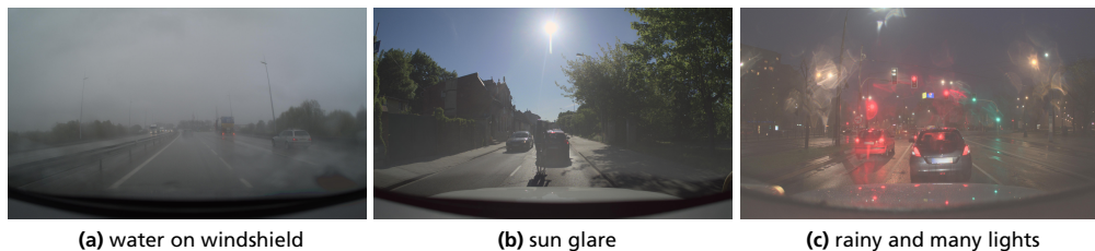
Figure 5.1: Heavy rain and strong sun glare, and the worst case when both are combined (headlights in heavy rain). These effects pose major difficulties for neural reconstruction methods like NeRFs and 3DGS.
