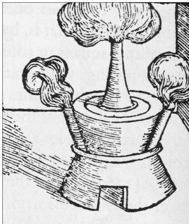
Fig. 7. Alundel, depicted in Biringuccio's Pyrotechnica from 1540. Source: Smith 1966: Fig. 69.
