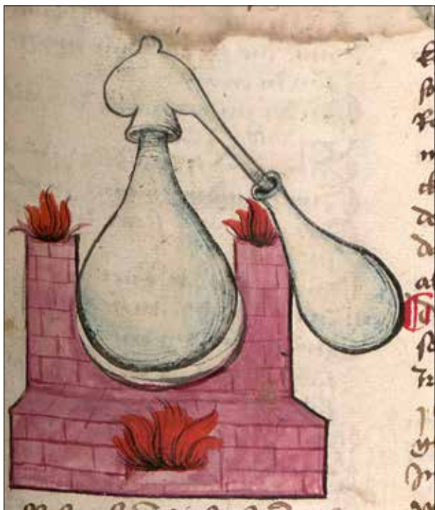
Fig. 6. Medieval depiction of a still consisting of a flask with an alembic, 2nd half 15th century. Source: Buch der heiligen Dreifaltigkeit – Bayerische Staatsbibliothek München Cgm 598.
