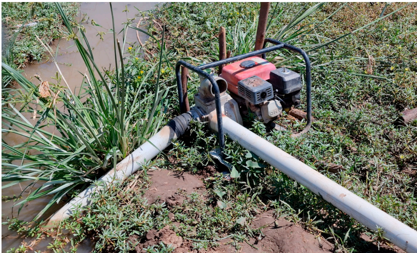
Image 18. Matthew's water pump sucking water from a man-made canal channeling water from Lake Baringo. He moves the pump as the water level rises and falls with the seasons. Photo: Osman Oleparmarin.
