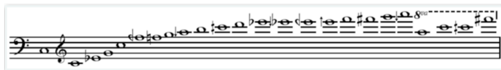
Figure 4.1, Spectrum of the tenor bell at Winchester Cathedral Analysed by Jonathan Harvey using FFT. In C. Roads (Ed.), The Music Machine (1992, p. 92)
