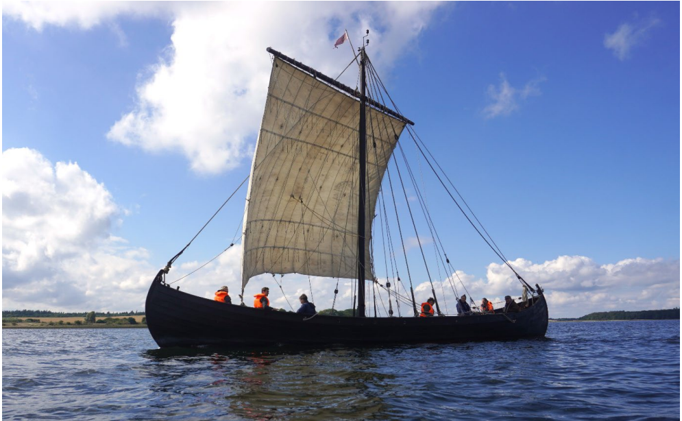
Supplementary Figure S2. Larger ‘expeditionary’ vessel employed by Greenland Norse. This modern example is a compact, clinker-built, square-rigged cargo vessel based on the design of the Skuldelev I wreck, which was built in western Norway c.1030 CE. Norse Greenlanders could only undertake walrus harvesting expeditions to the North Water Polynya in these larger sailing vessels, which were owned by wealthier farmers and elites, adding an important socio-political dimension to Late Period exploitation strategies. Photo: Greer Jarrett.
