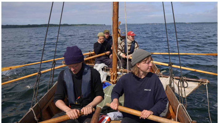
Fig. 3. Experimental insights into Greenland Norse seafaring capabilities: example of a “smaller” vessel (with oars and sail). This is a Norwegian firing during sea trials. Note the very limited space for cargo (Roskilde Fjord, Denmark, June 2023). Photo: G.J.
