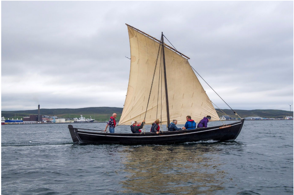
Supplementary Figure S1. Smaller vessel employed by Greenland Norse. The Shetland sixareen (pictured) is probably the most similar surviving relative of the smaller six-oared boats used by the Greenland Norse, although such boats would have carried a square rather than a lug sail. Such boats would have been used to harvest local walrus stocks but were not suitable for the High Arctic expeditions to the North Water Polynya. Photo: Dave Donaldson (reproduced with permission).
