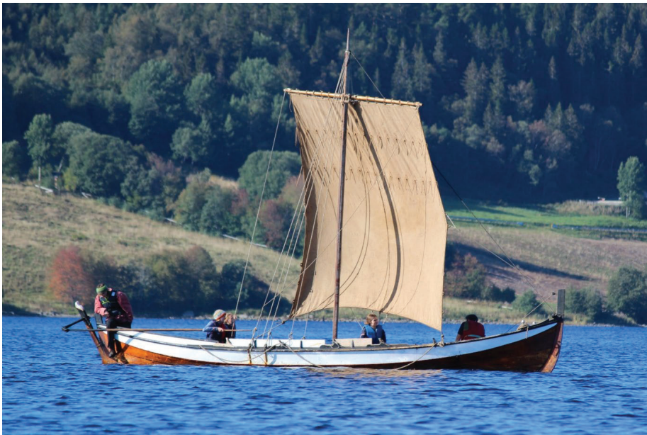
Fig. 3 Continuities in boatbuilding traditions from the Viking Age are evident in the shape and rig of this fying , a smaller type of Åfjord boat similar to the vessels associated with non-elite Viking Age farmsteads. Image courtesy of Tora Heide
