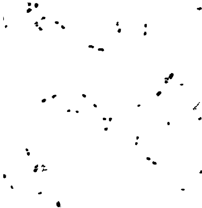
Figure 21. Successful differential image of HDM moving on a Petri dish. Each moving HDM is represented by two dots.
