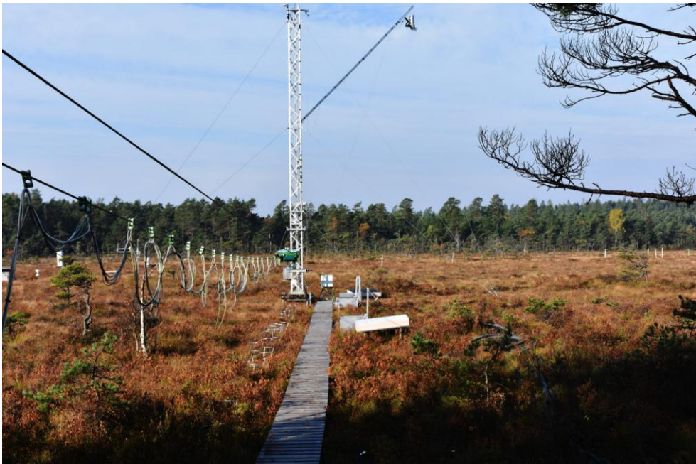
Figure8. Mycklemossen Mire measurement site within the Skogaryd Research Catchment, southwestern Sweden. Mycklemossen is part of the SITES infrastructure and an ICOS Ecosystem Station (SE-Myc), where continuous GHG fluxes are measured using an EC tower. The site is also equipped with automatic chamber systems.
