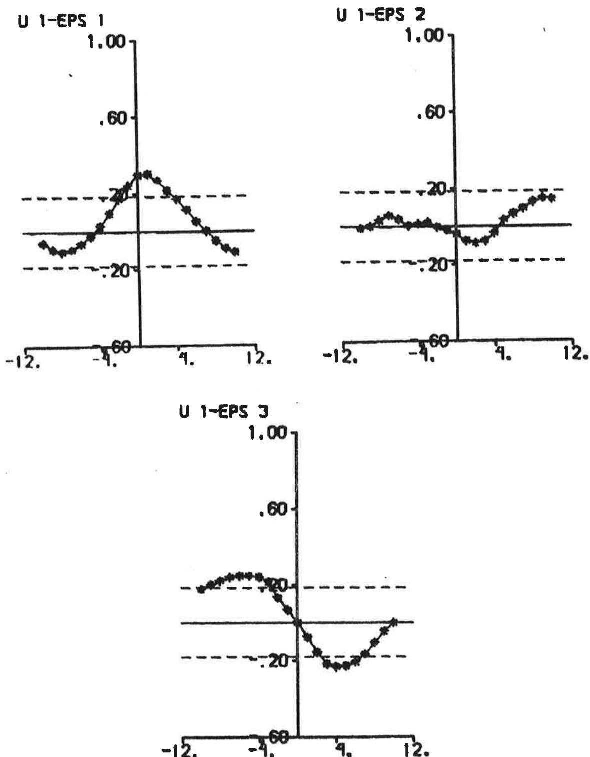
Fig. 4.10d - Cross correlation functions between rudder input and prediction errors.
