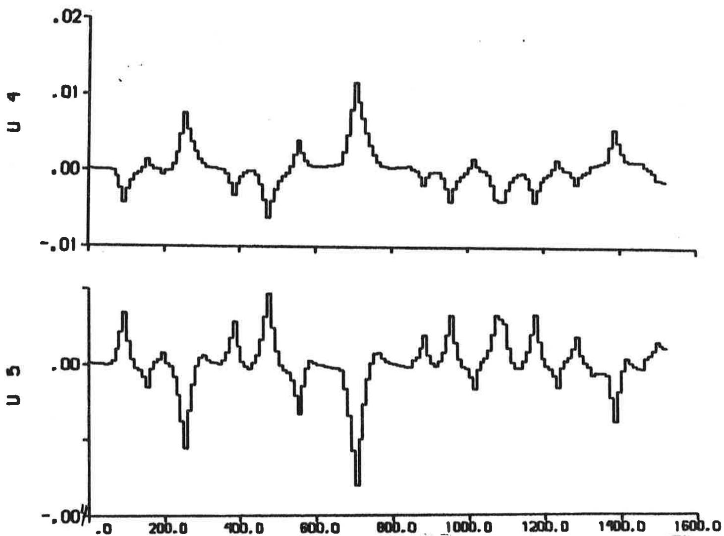
Fig. 5.10b - Additional inputs  $U_4 = f_Y/m'$  and  $U_5 = f_N/m'$  describing the nonlinear contributions.
