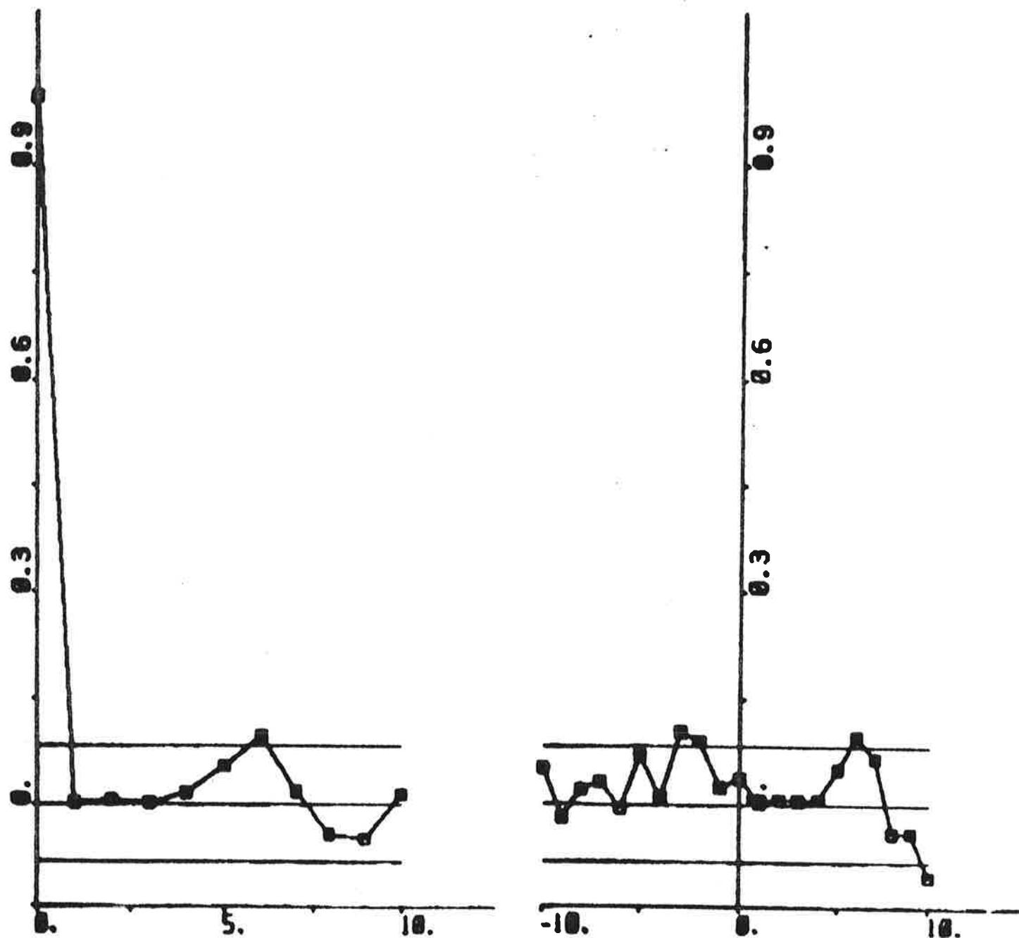
Fig. 6.56 - Autocorrelation function of residuals and cross correlation function between rudder input and residuals, where the residuals are obtained from ML identification using IDPAC to data from experiment E3 (4th order model).
