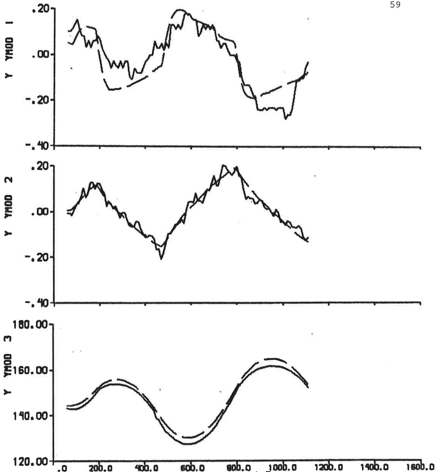
Fig. 4.10a - Result of prediction error identification ( $p = 6$ ) to data from experiment E2. The rudder angle is the input signal.
