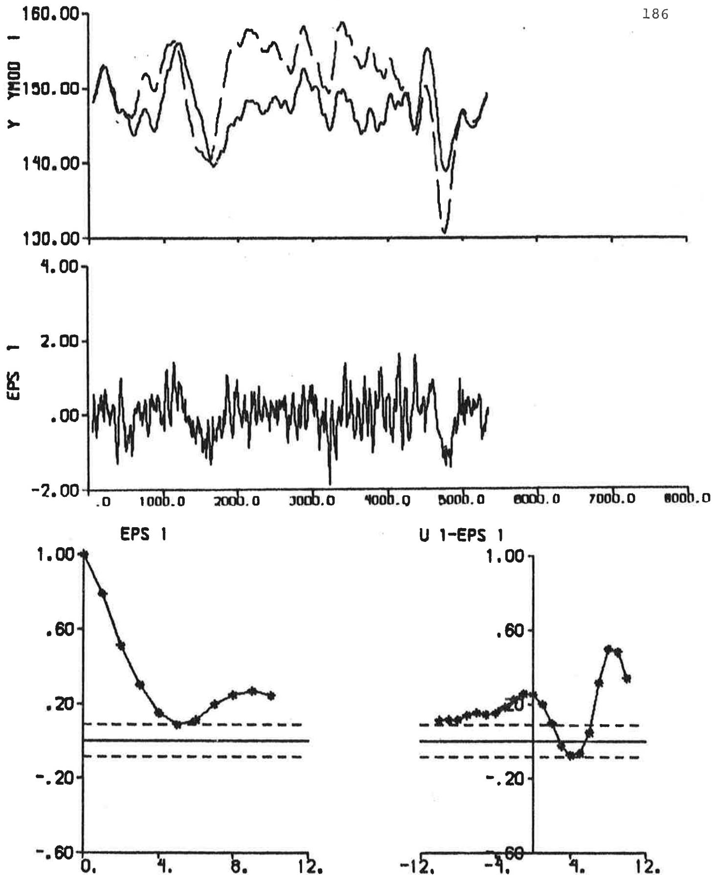
Fig. 6.34 - Result of prediction error identification ( $p = 6$ ) to data from experiment El. Nomoto's model is used and the rudder angle is the input signal.
