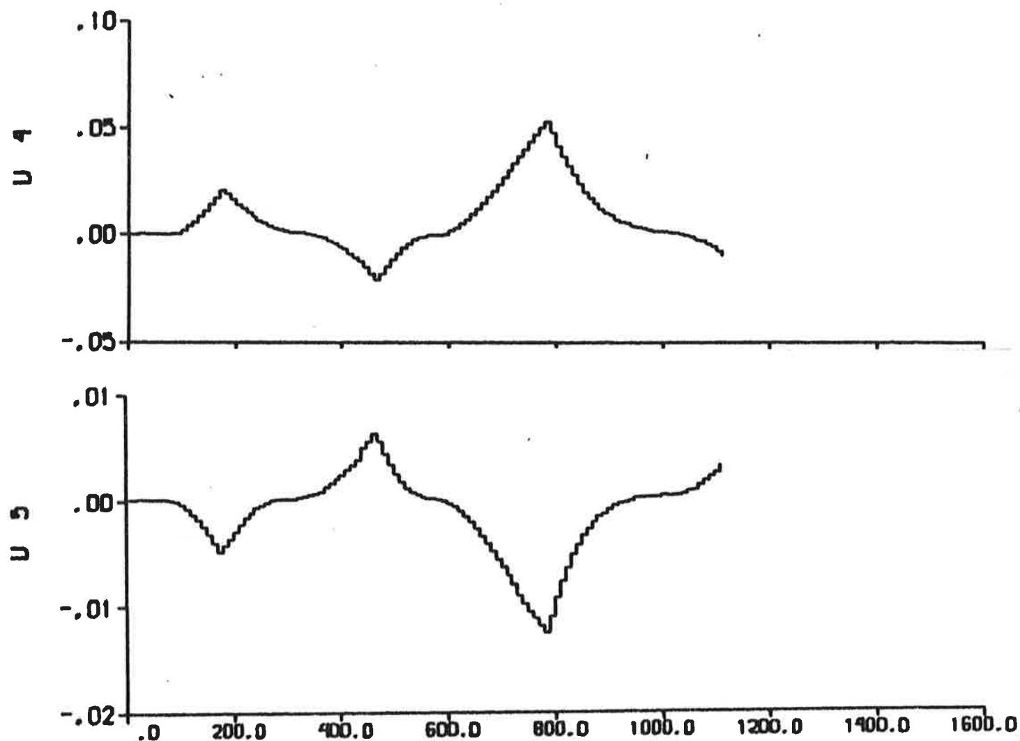
Fig. 5.6b - Additional inputs  $U_4 = f_Y/m'$  and  $U_5 = f_N/m'$  describing the nonlinear contributions.
