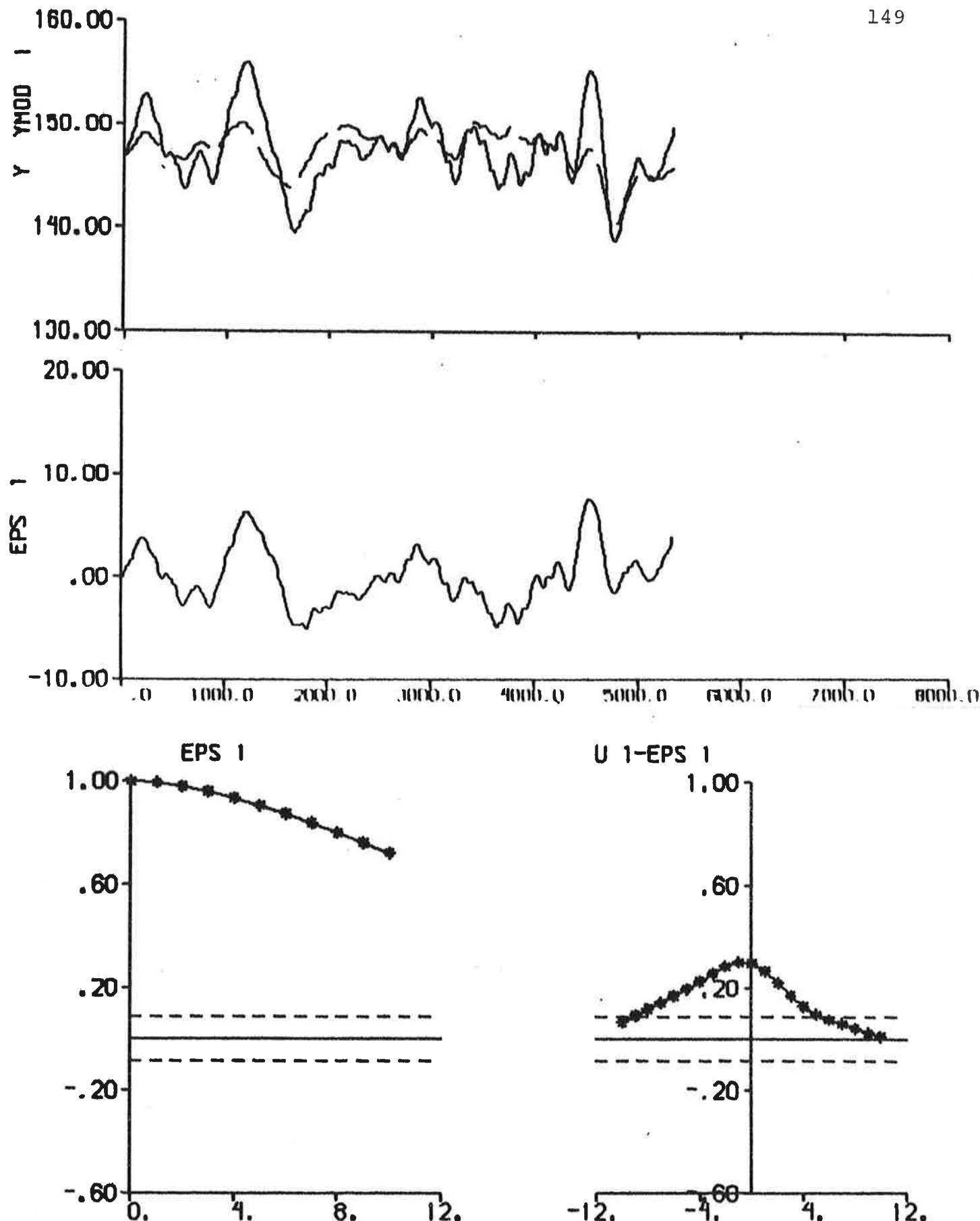
Fig. 6.1 - Result of output error identification to data from experiment El.
