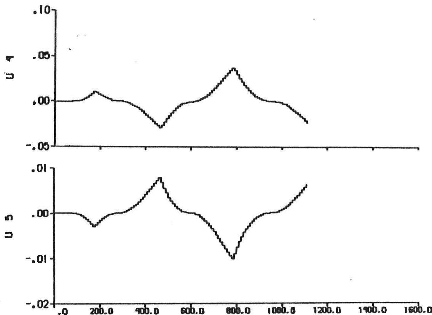
Fig. 5.14b - Additional inputs  $U_4 = f_Y/m'$  and  $U_5 = f_N/m'$  describing the nonlinear contributions.
