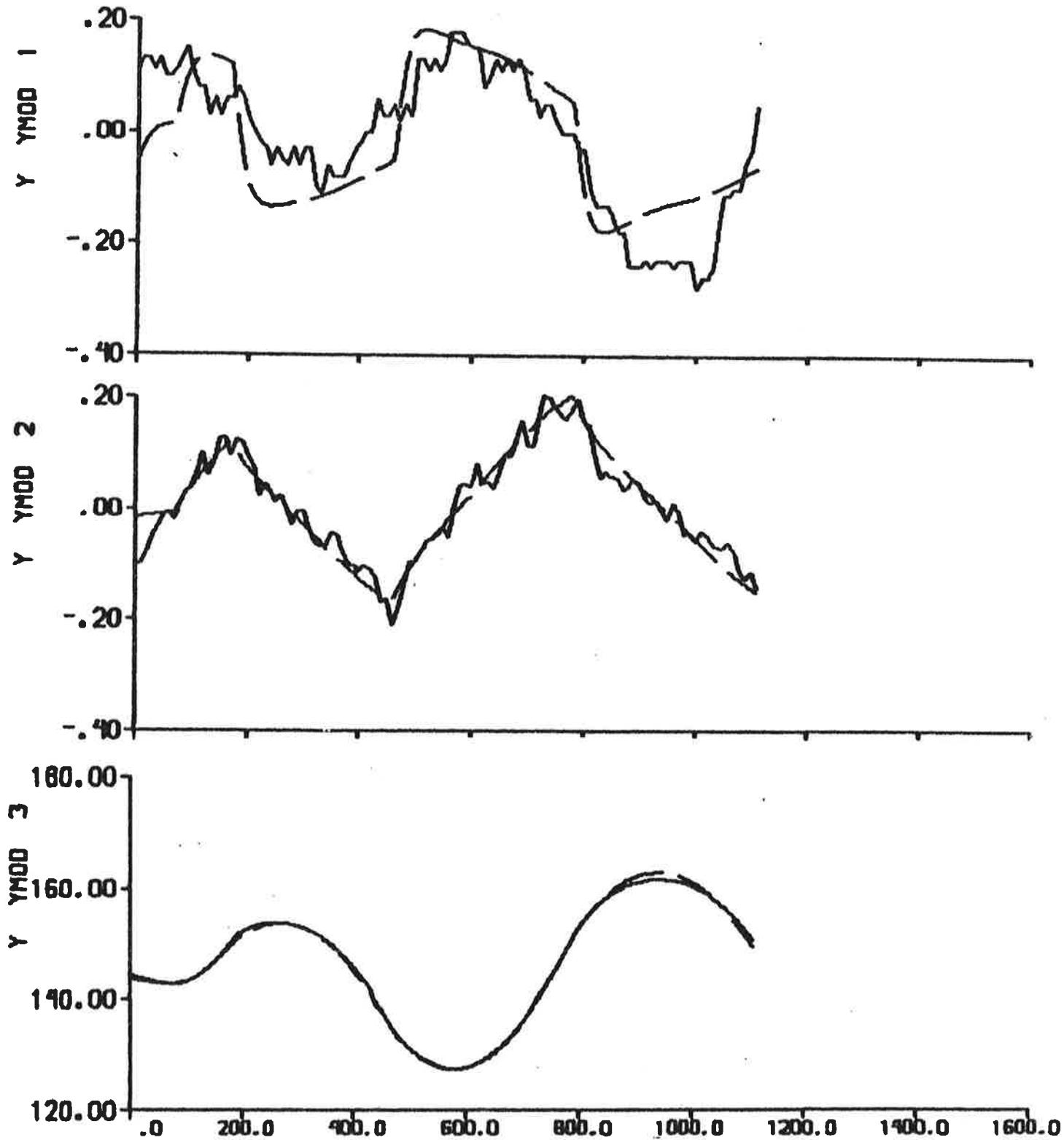
Fig. 5.14a - Result of output error identification to data from experiment E2, when the model is fixed to the model obtained from prediction error identification ( $p = 6$ ) to data from E2.  $C = 0.63$ .
