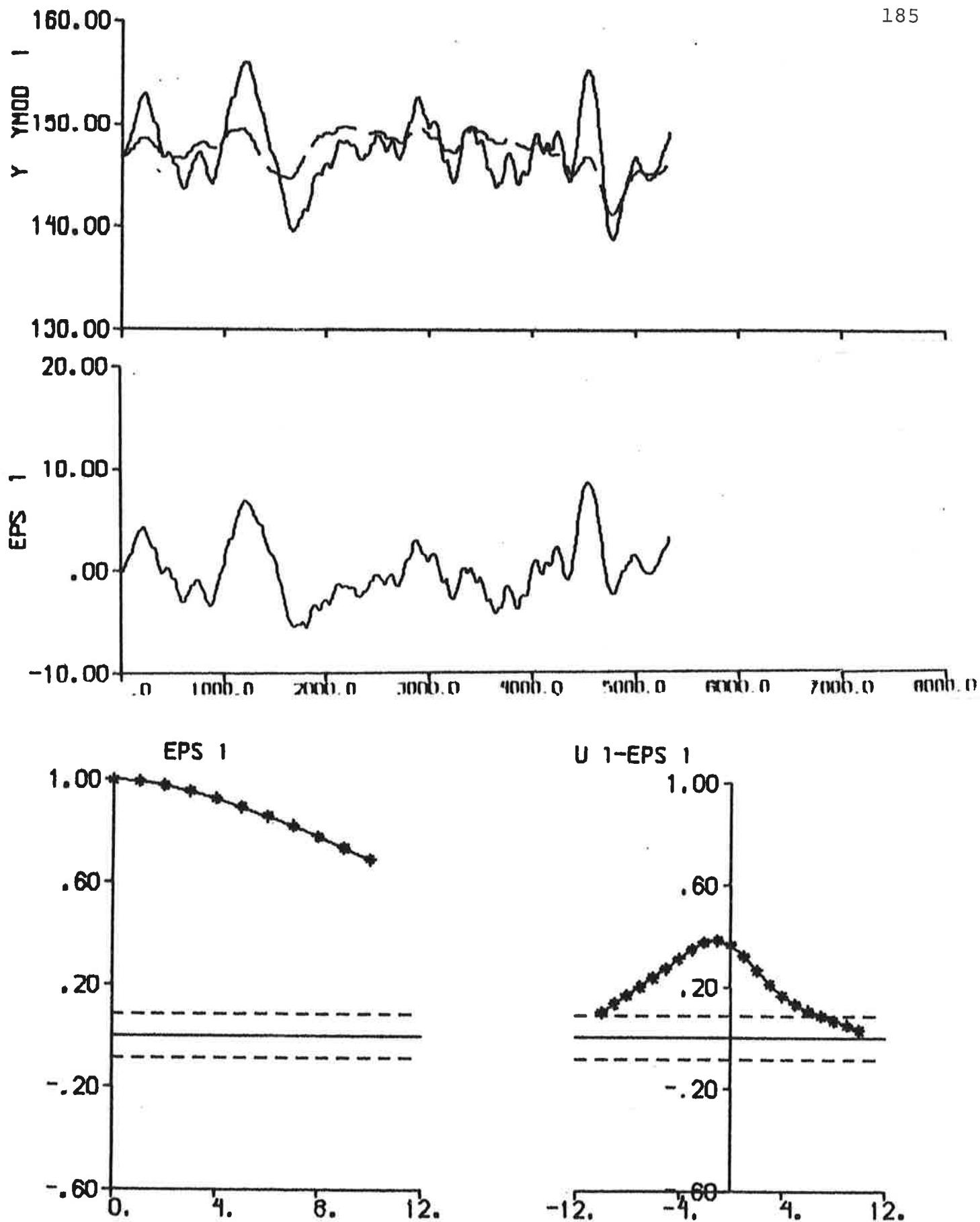
Fig. 6.33 - Result of output error identification to data from experiment El. Nomoto's model is used and the rudder angle is the input signal.
