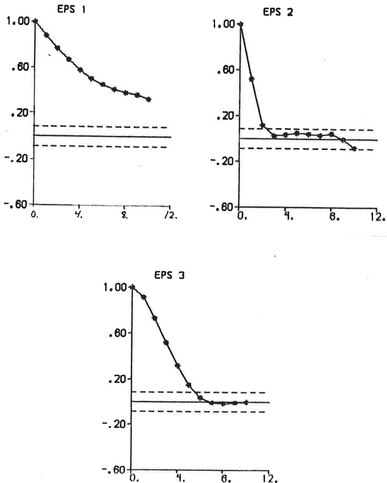
Fig. 4.15c - Autocorrelation functions of prediction errors.
