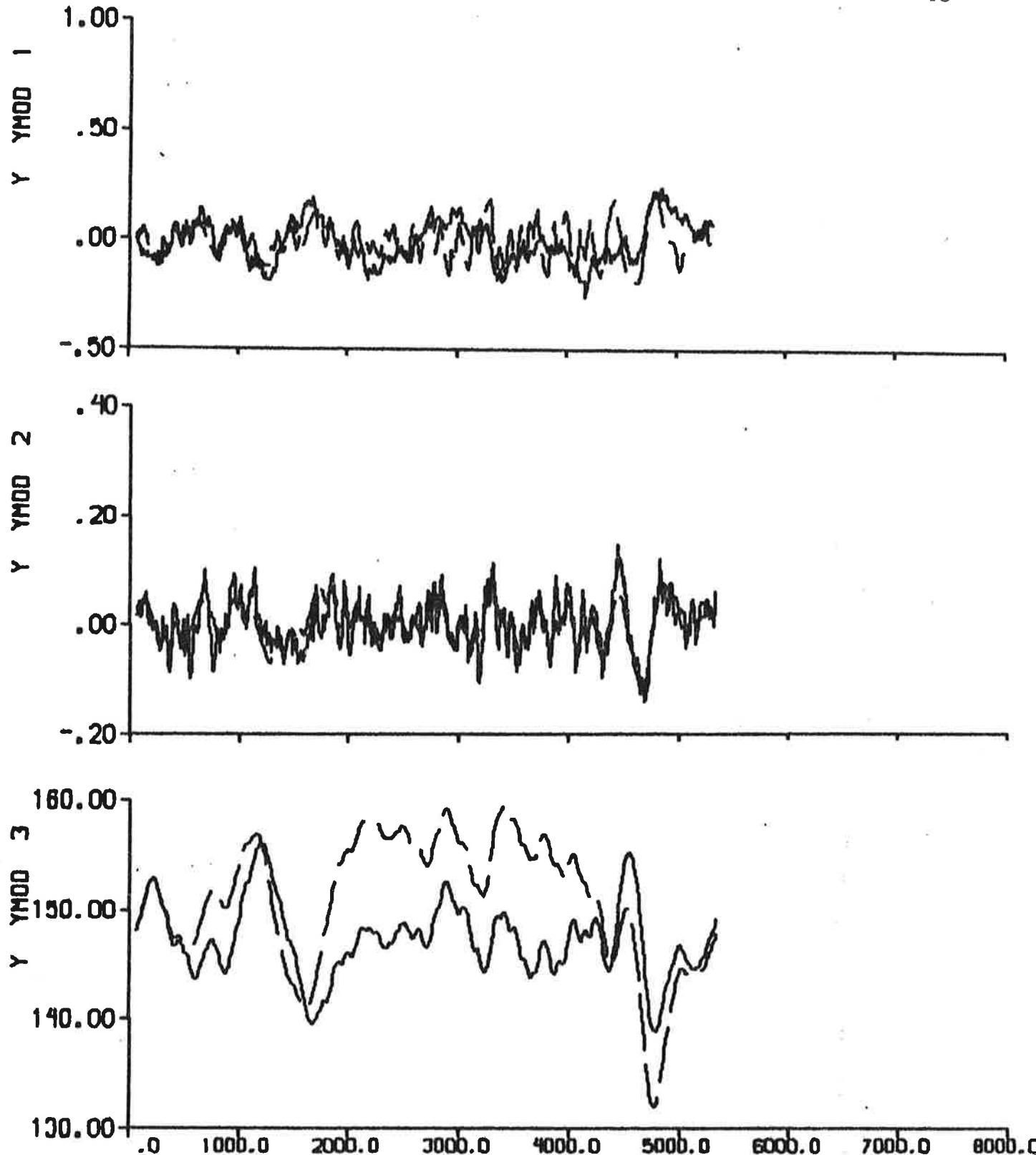
Fig. 4.5a - Result of prediction error identification ( $p = 6$ ) to data from experiment El. The rudder angle is the input signal.
