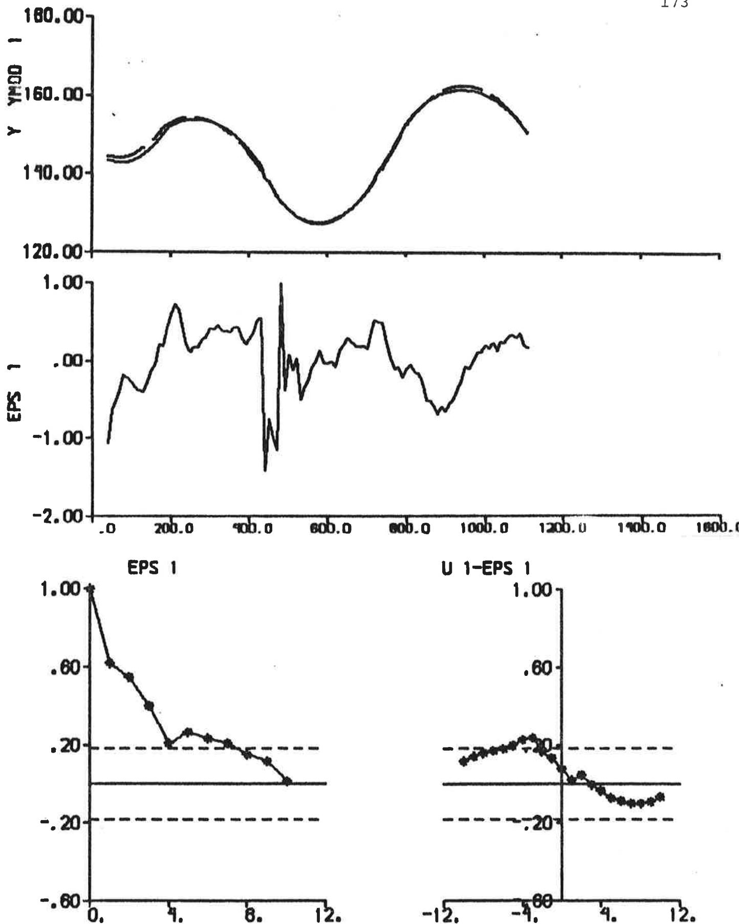
Fig. 6.23 - Result of prediction error identification ( $p = 4$ ) to data from experiment E2.
