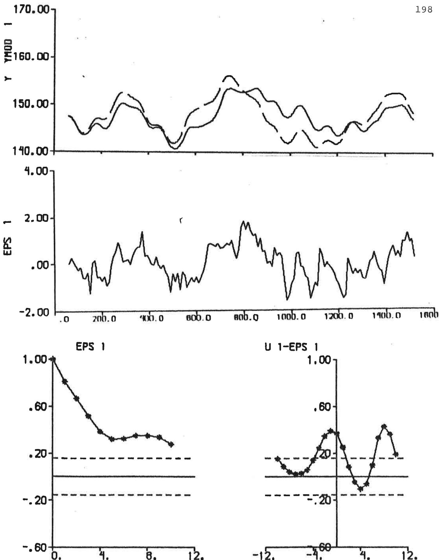
Fig. 6.46 - Result of prediction error identification ( $p = 6$ ) to data from experiment E4. Nomoto's model is used and the rudder angle is the input signal.
