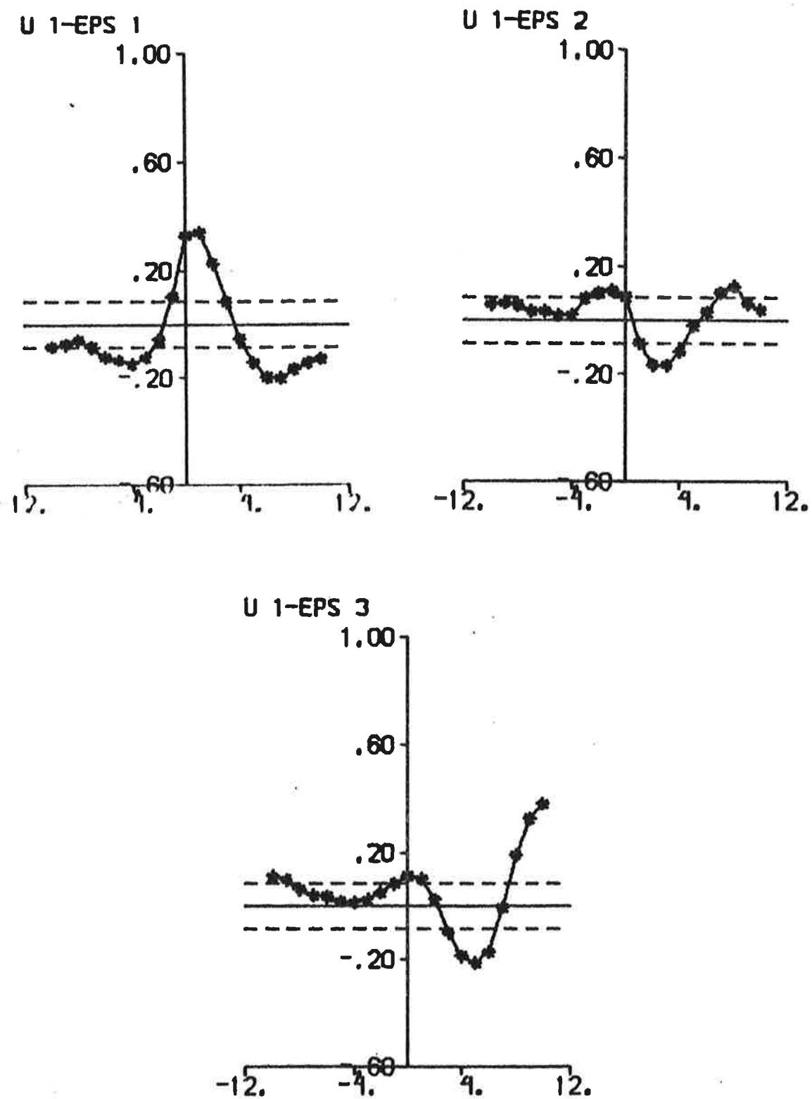
Fig. 5.3e - Cross correlation functions between rudder input and prediction errors.
