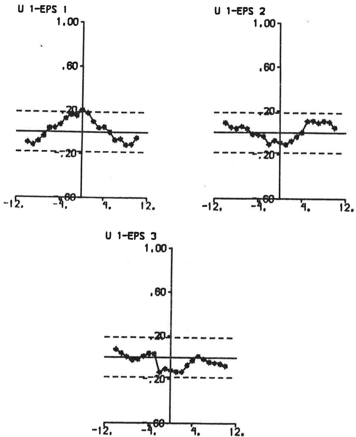
Fig. 4.8d - Cross correlation functions between rudder input and prediction errors.
