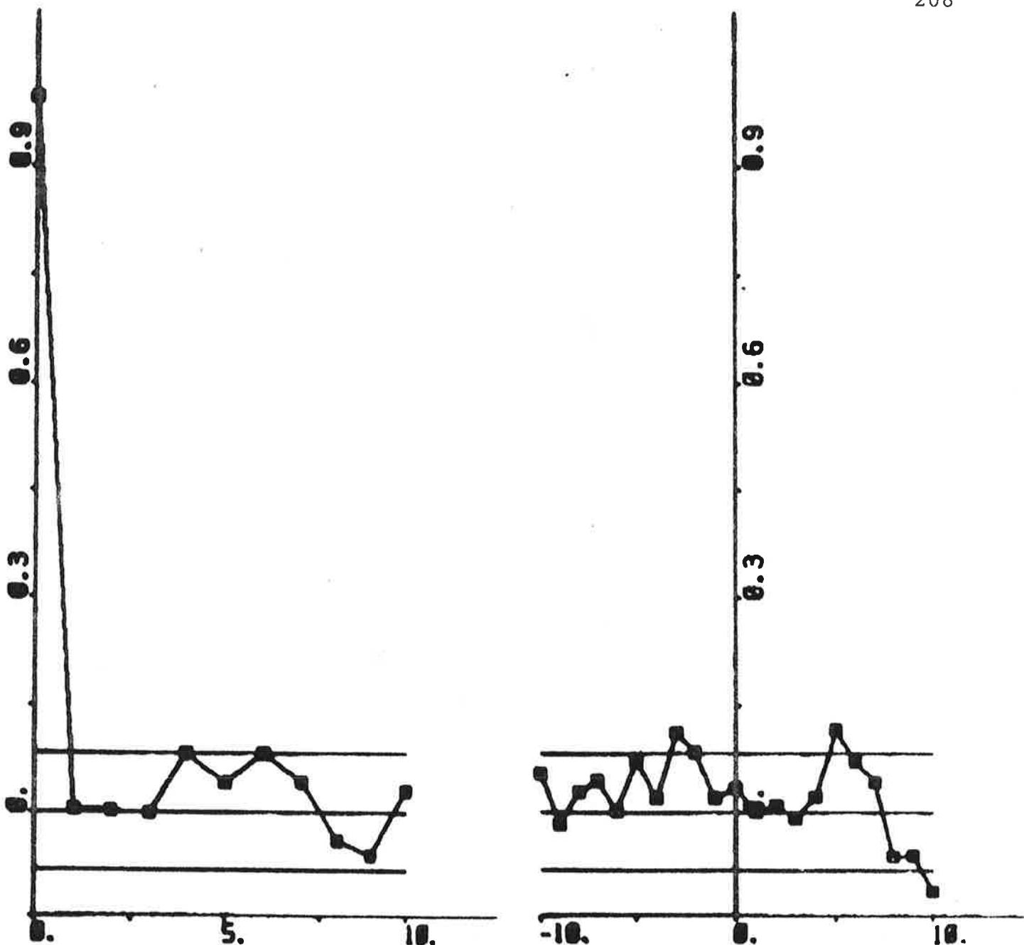
Fig. 6.52 - Autocorrelation function of residuals and cross correlation function between rudder input and residuals, where the residuals are obtained from ML identification using IDPAC to data from experiment E3 ( $b_3$  estimated).
