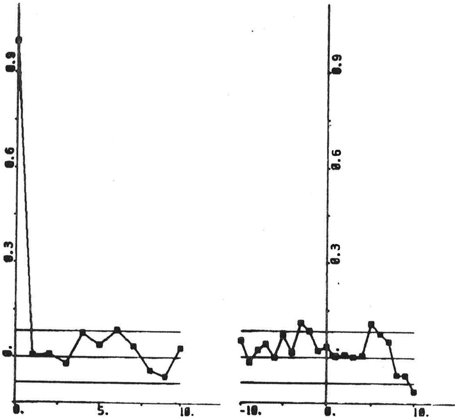
Fig. 6.55 - Autocorrelation function of residuals and cross correlation function between rudder input and residuals, where the residuals are obtained from ML identification using IDPAC to data from experiment E3 (3rd order model).
