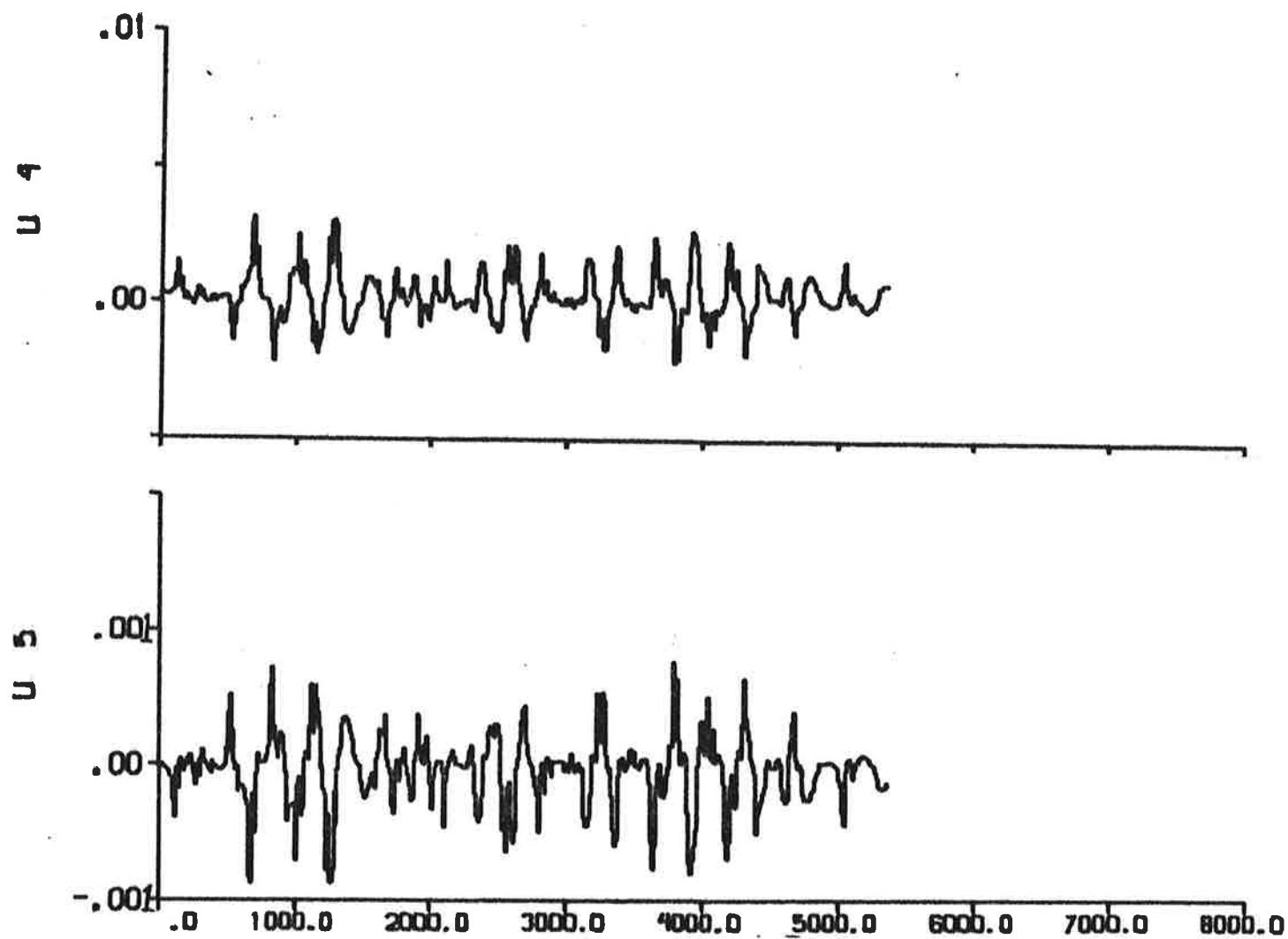
Fig. 5.7b - Additional inputs  $U_4 = f_Y/m'$  and  $U_5 = f_N/m'$  describing the nonlinear contributions.
