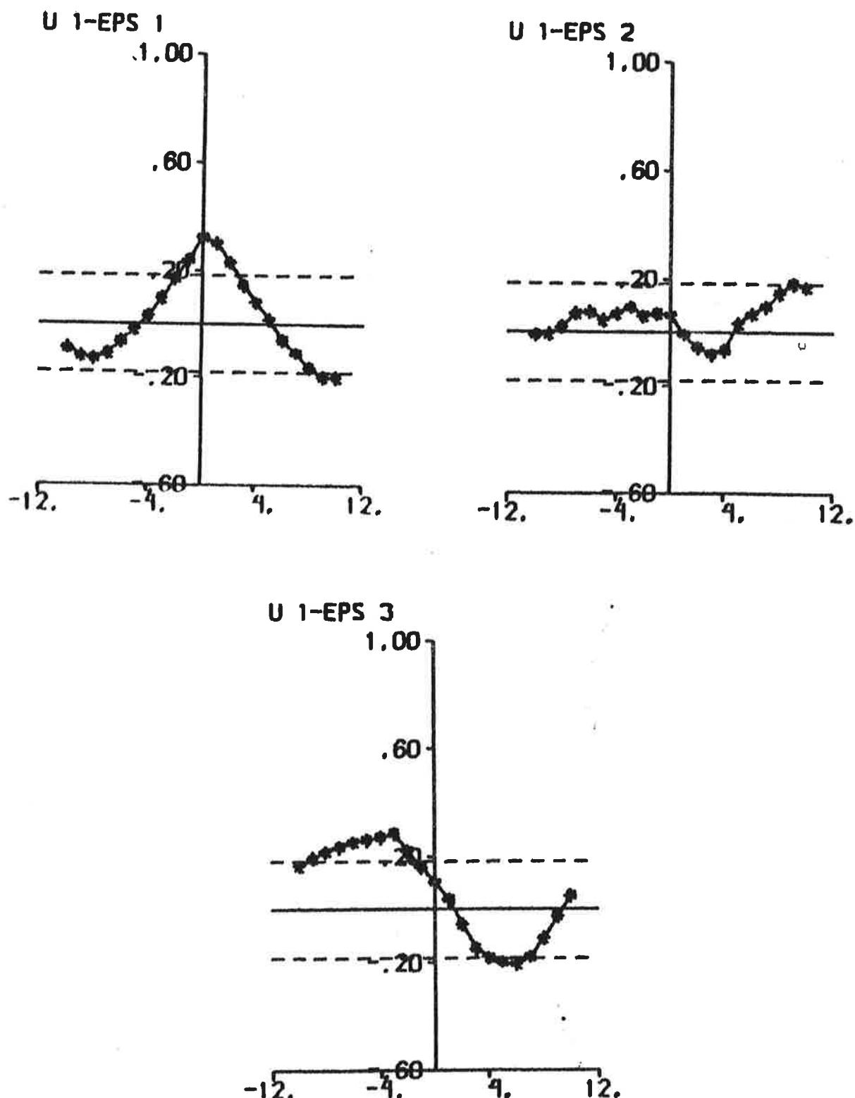
Fig. 5.6e - Cross correlation functions between rudder input and prediction errors.
