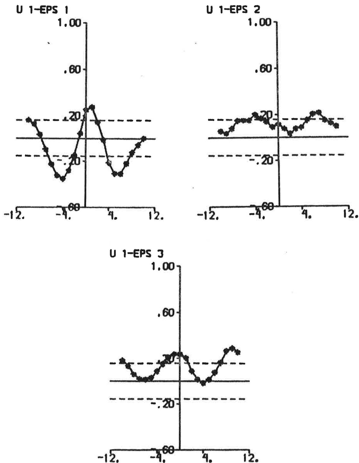
Fig. 4.19d - Cross correlation functions between rudder input and prediction errors.
