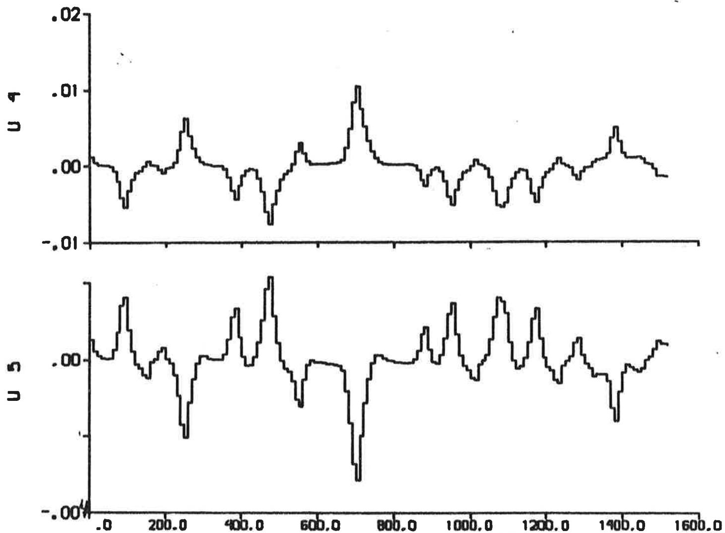
Fig. 5.11b - Additional inputs  $U_4 = f_Y/m'$  and  $U_5 = f_N/m'$  describing the nonlinear contributions.
