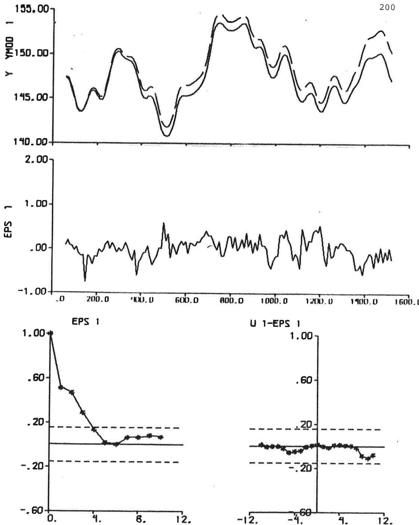
Fig. 6.48 - Result of prediction error identification ( $p = 6$ ) to data from experiment E4. The transfer function (3.12) is used and the rudder angle is the input signal.
