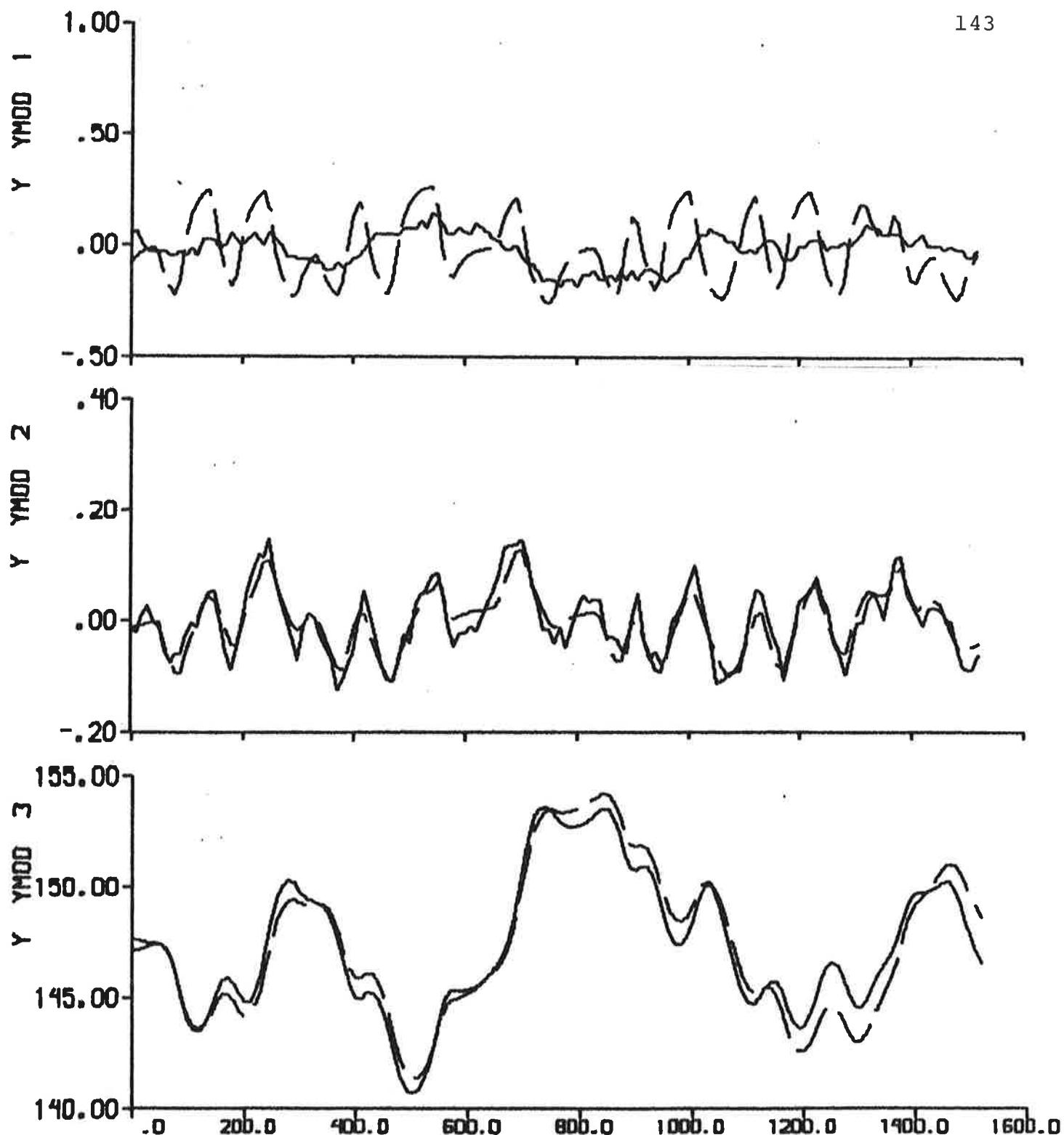
Fig. 5.18a - Result of output error identification to data from experiment E4, when the model is fixed to the model obtained from prediction error identification ( $p = 6$ ) to data from E2. C is estimated.
