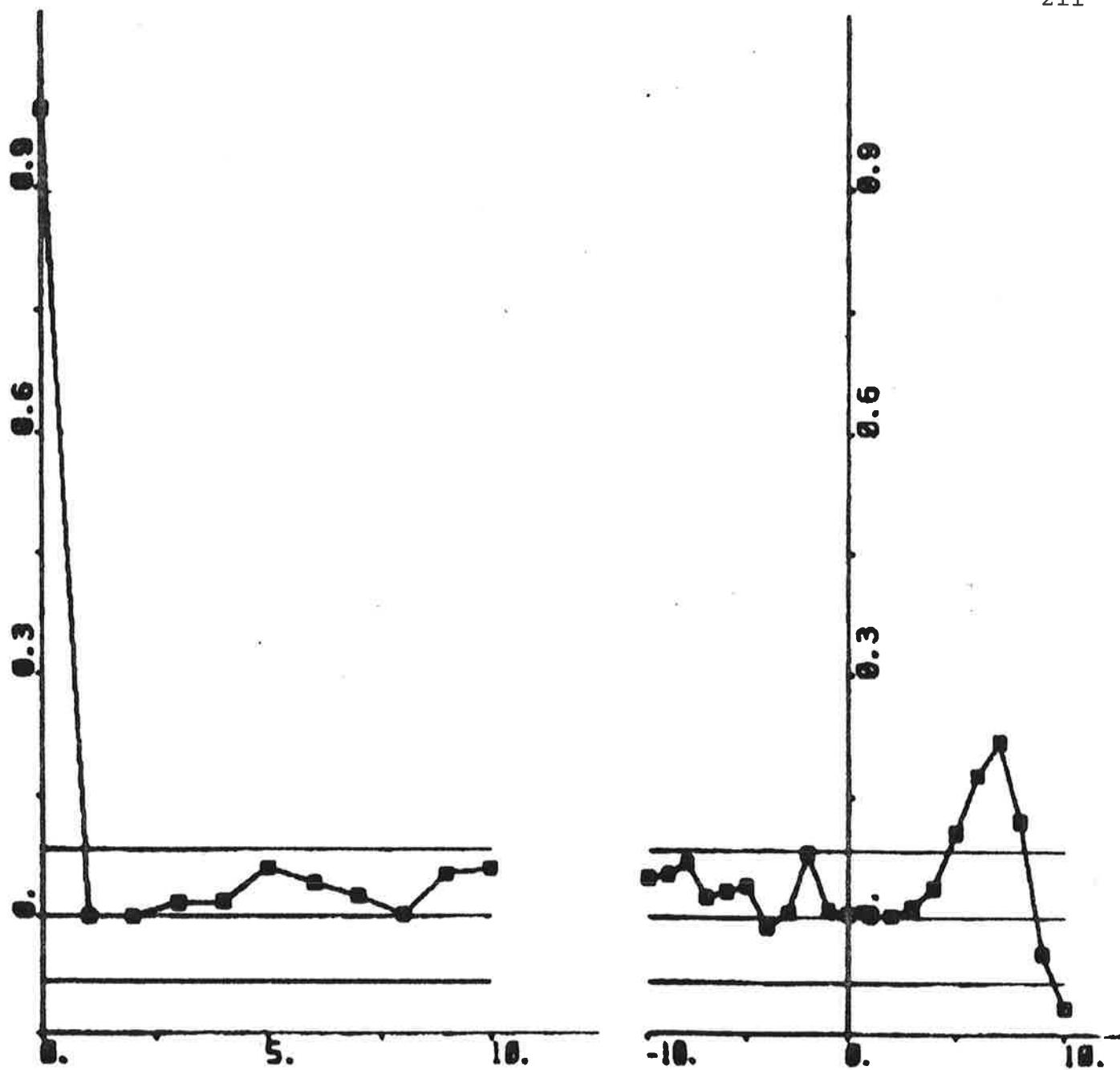
Fig. 6.54 - Autocorrelation function of residuals and cross correlation function between rudder input and residuals, where the residuals are obtained from ML identification using IDPAC to data from experiment El (4th order model).
