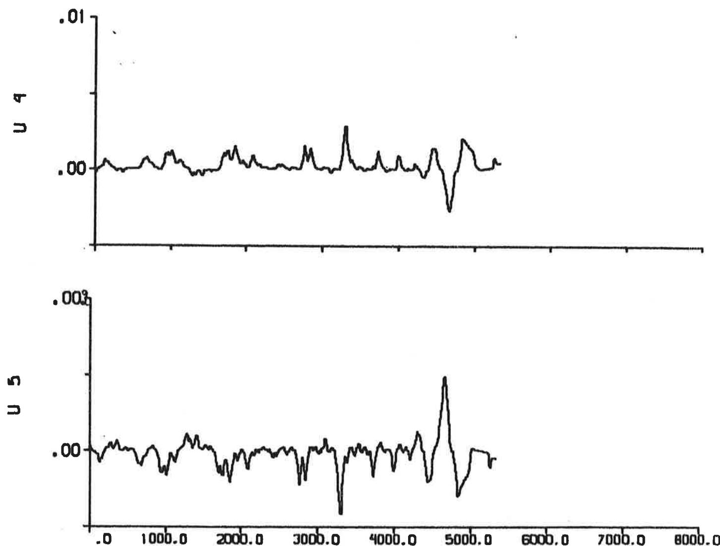
Fig. 5.2b - Additional inputs  $U_4 = f_Y/m'$  and  $U_5 = f_N/m'$  describing the nonlinear contributions.
