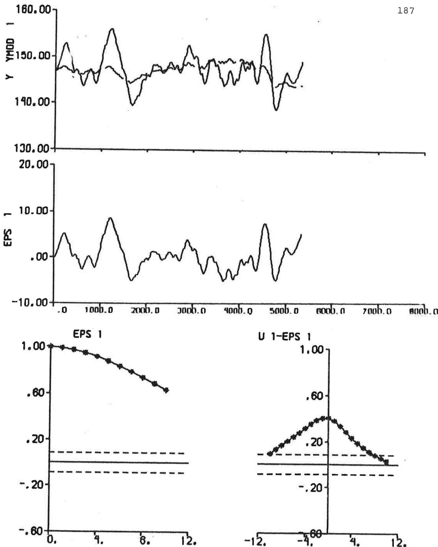
Fig. 6.35 - Result of output error identification to data from experiment El. The transfer function (3.12) is used and the rudder angle is the input signal.
