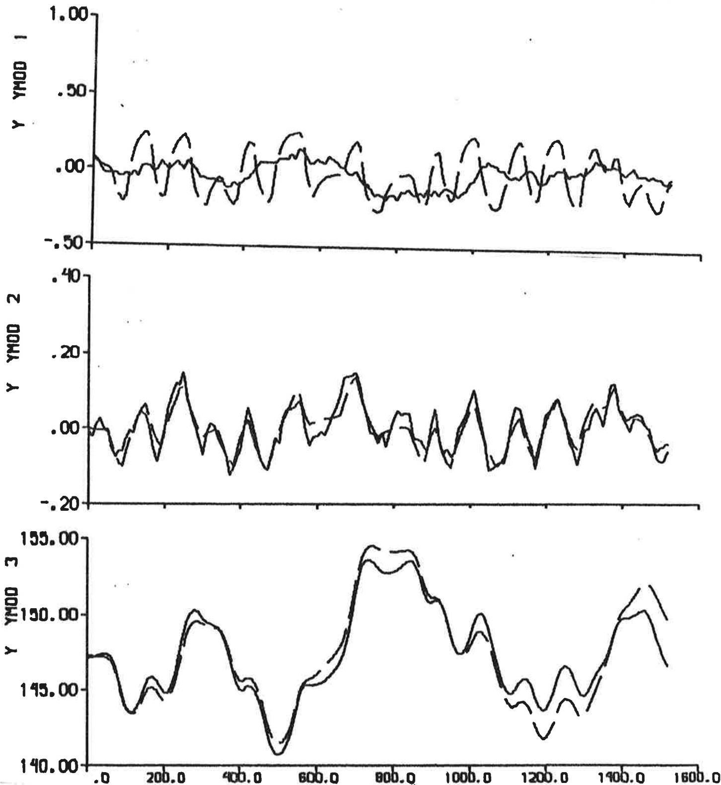
Fig. 5.17a - Result of output error identification to data from experiment E4, when the model is fixed to the model obtained from prediction error identification ( $p = 6$ ) to data from E2.  $C = 0.63$ .
