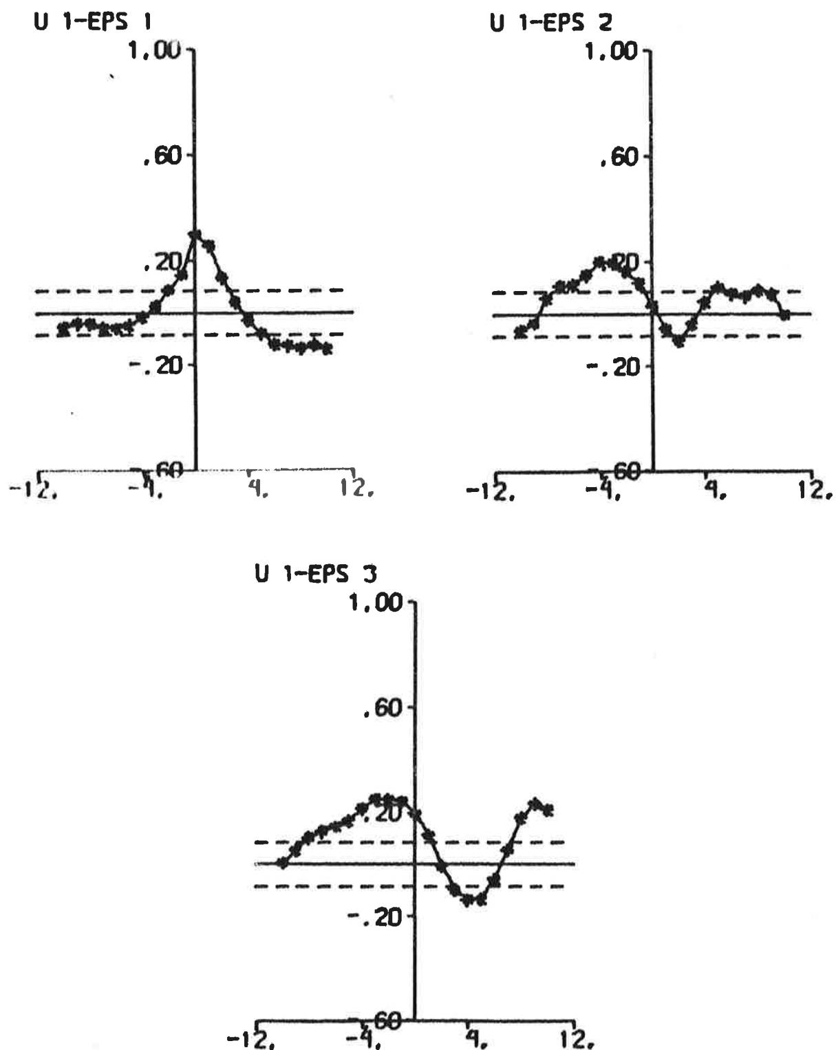
Fig. 5.9e - Cross correlation functions between rudder input and prediction errors.
