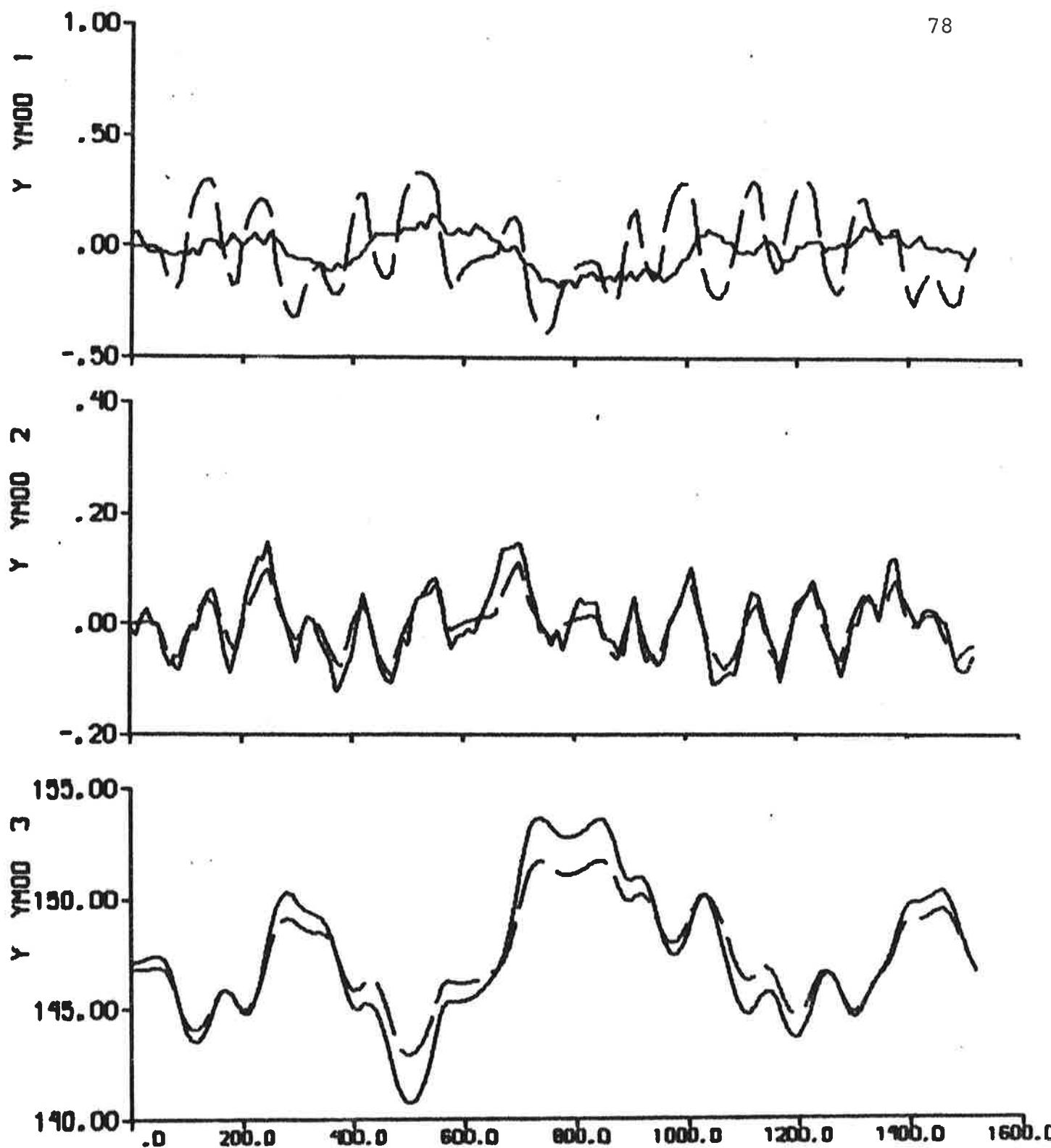
Fig. 4.16 - Result of output error identification to data from experiment E4, when the model is fixed to SSPA:s model.
