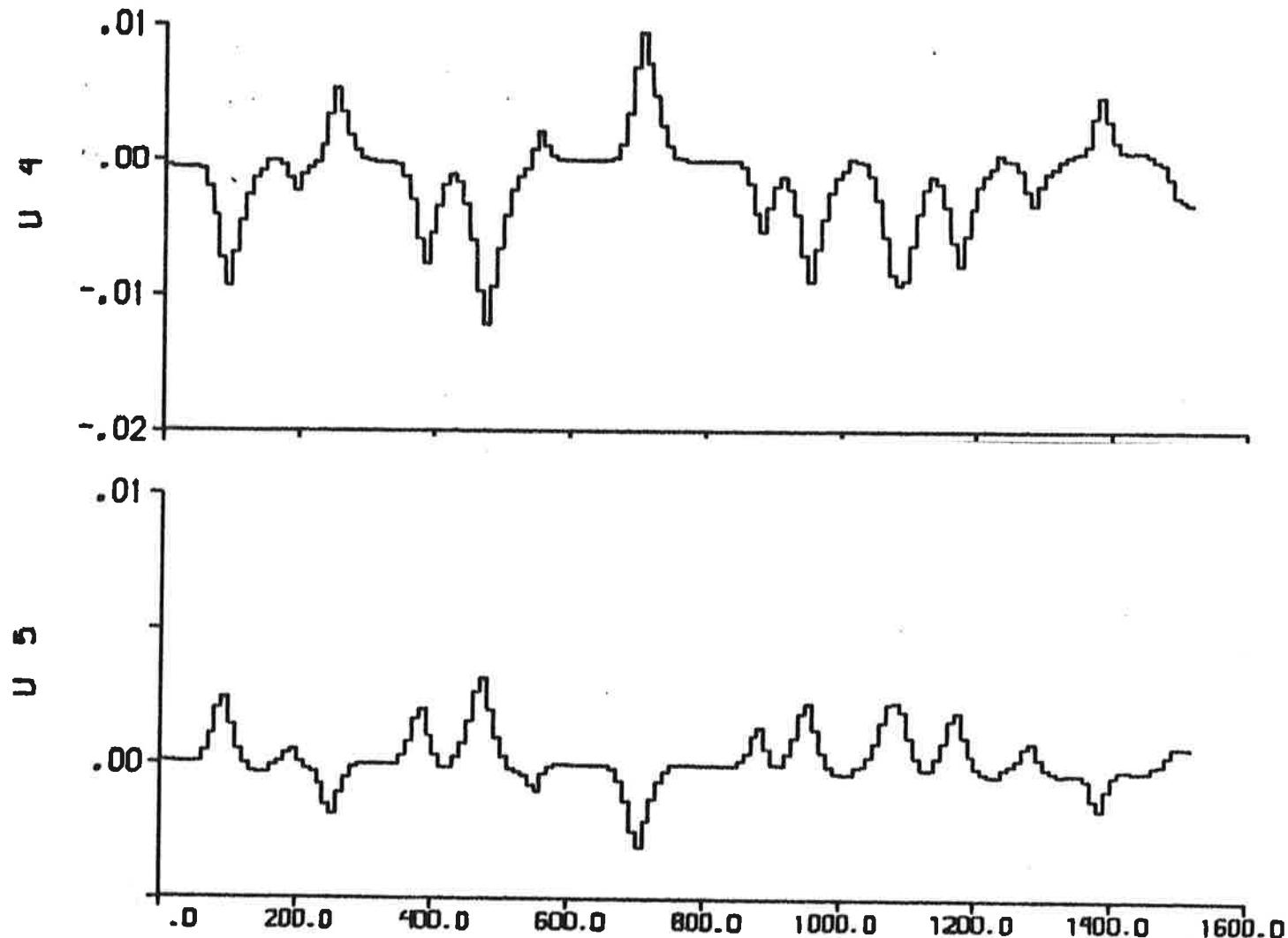
Fig. 5.18b - Additional inputs  $U_4 = f_Y/m'$  and  $U_5 = f_N/m'$  describing the nonlinear contributions.
