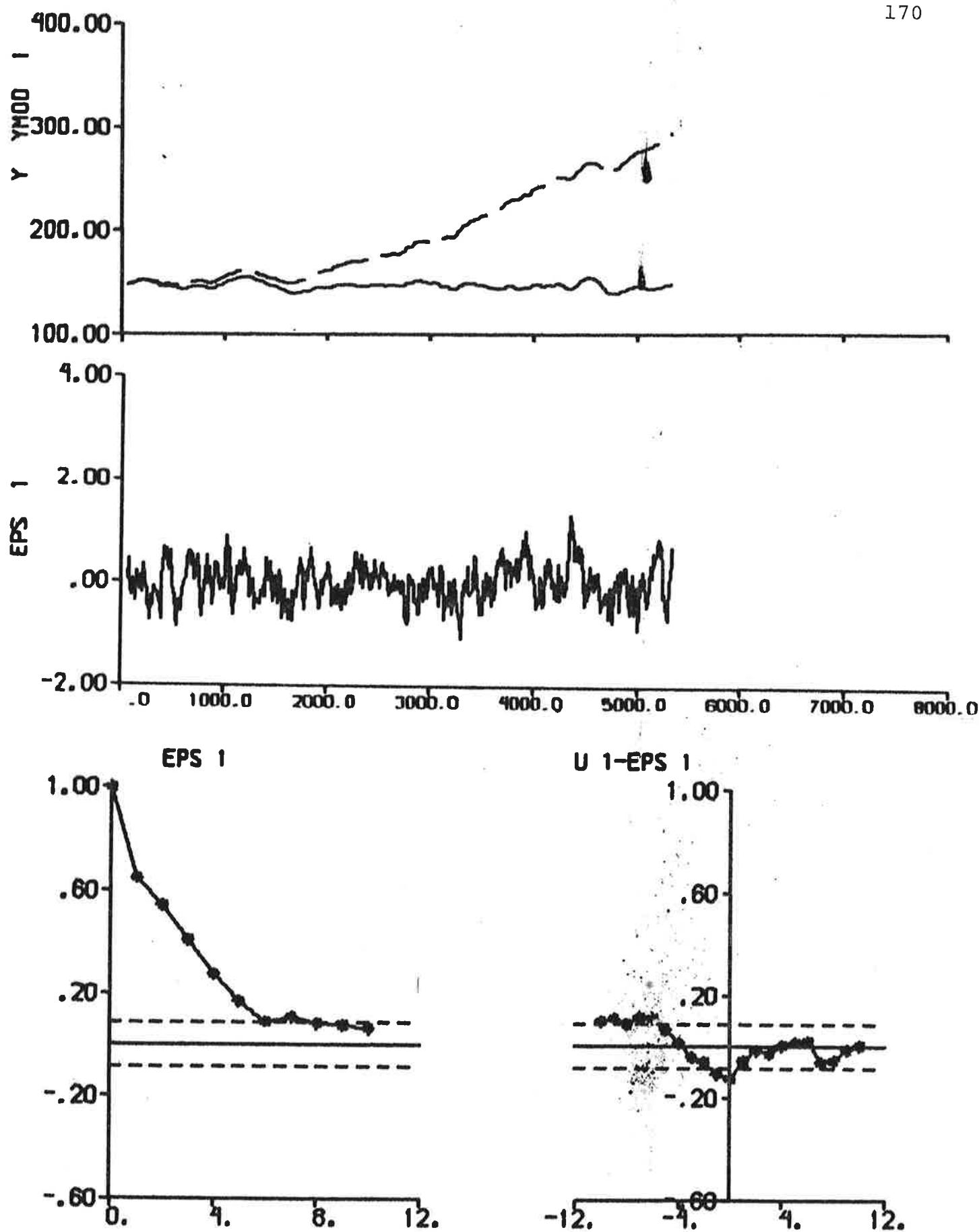
Fig. 6.20 - Result of prediction error identification ( $p = 6$ ) to data from experiment El.
