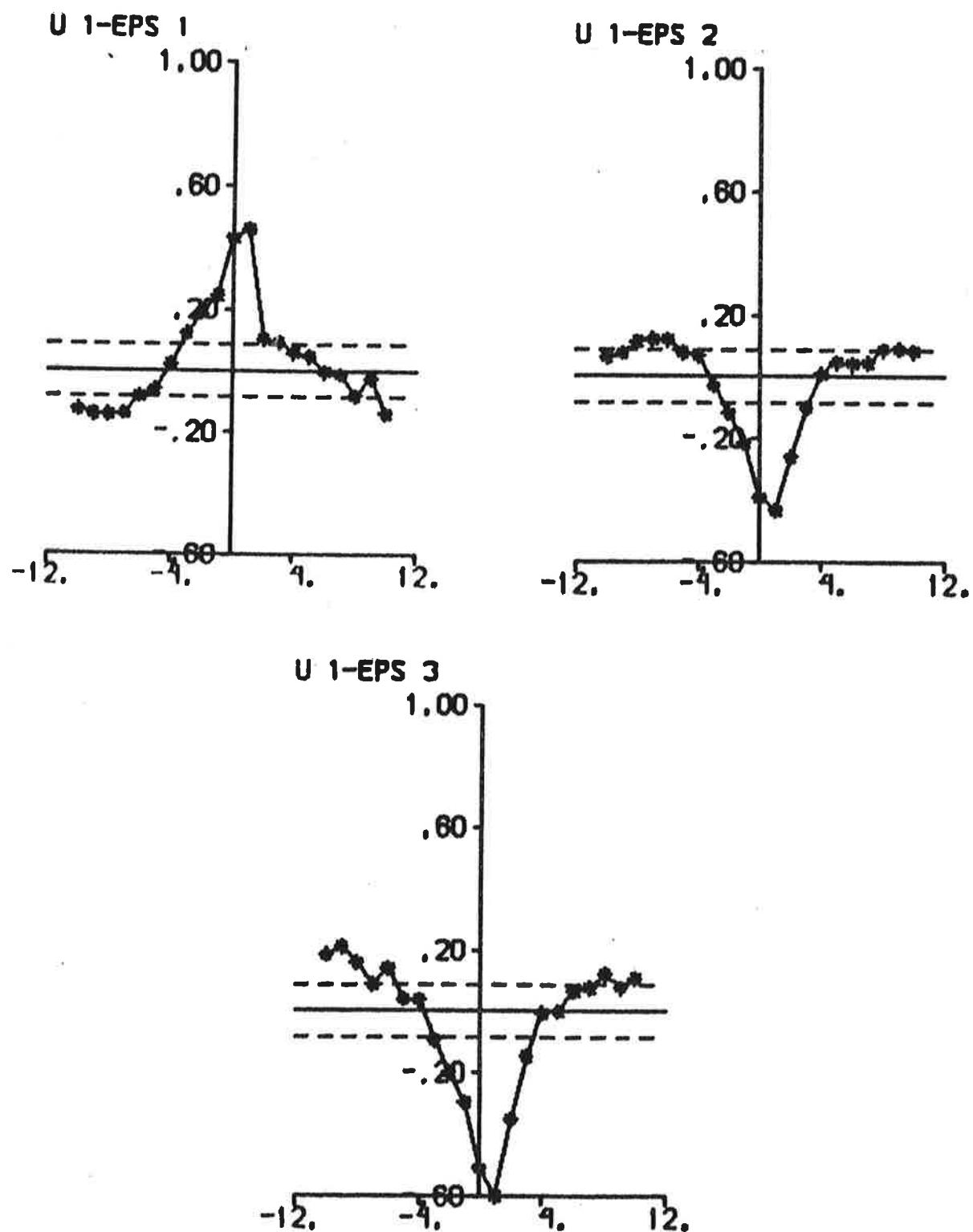
Fig. 4.13d - Cross correlation functions between rudder input and prediction errors.
