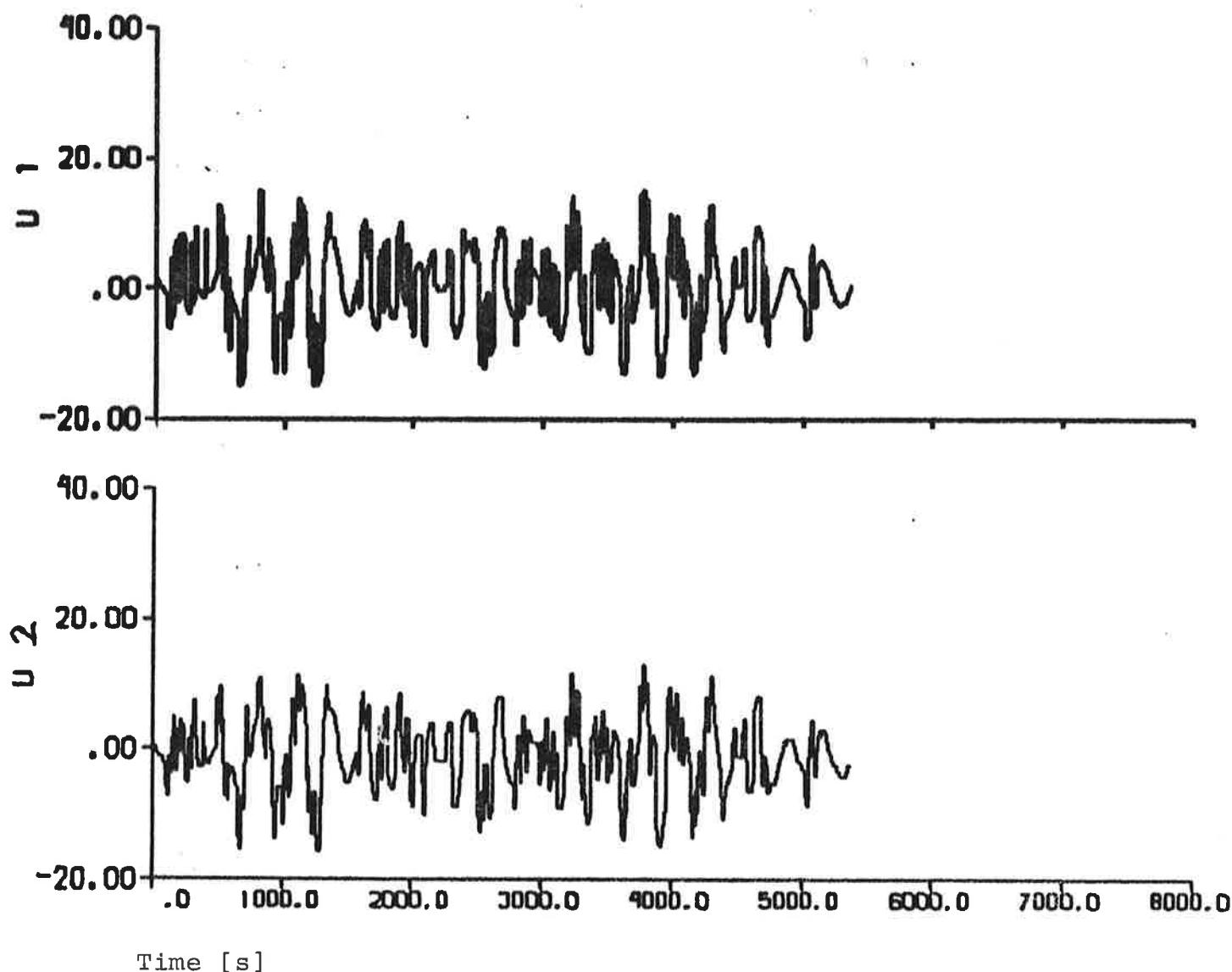
Fig. 2.3a - Input - output data obtained from experiment E3.
