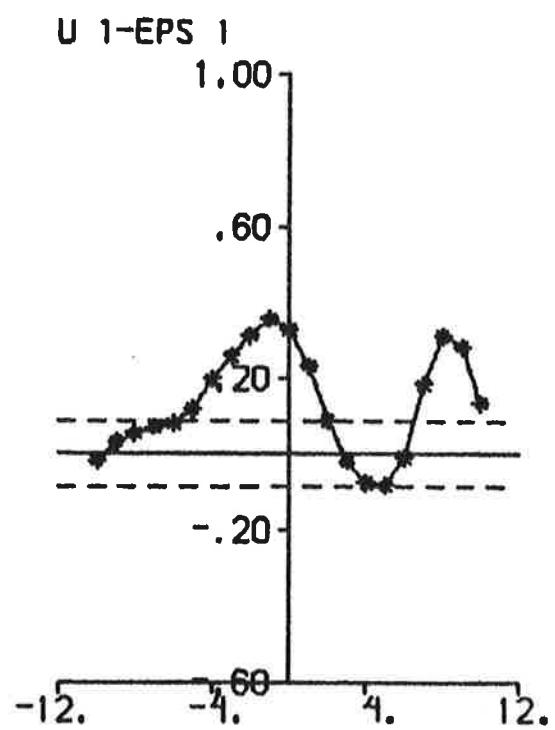
Fig. 6.42 - Result of prediction error identification ( $p = 6$ ) to data from experiment E3. Nomoto's model is used and the rudder angle is the input signal.
