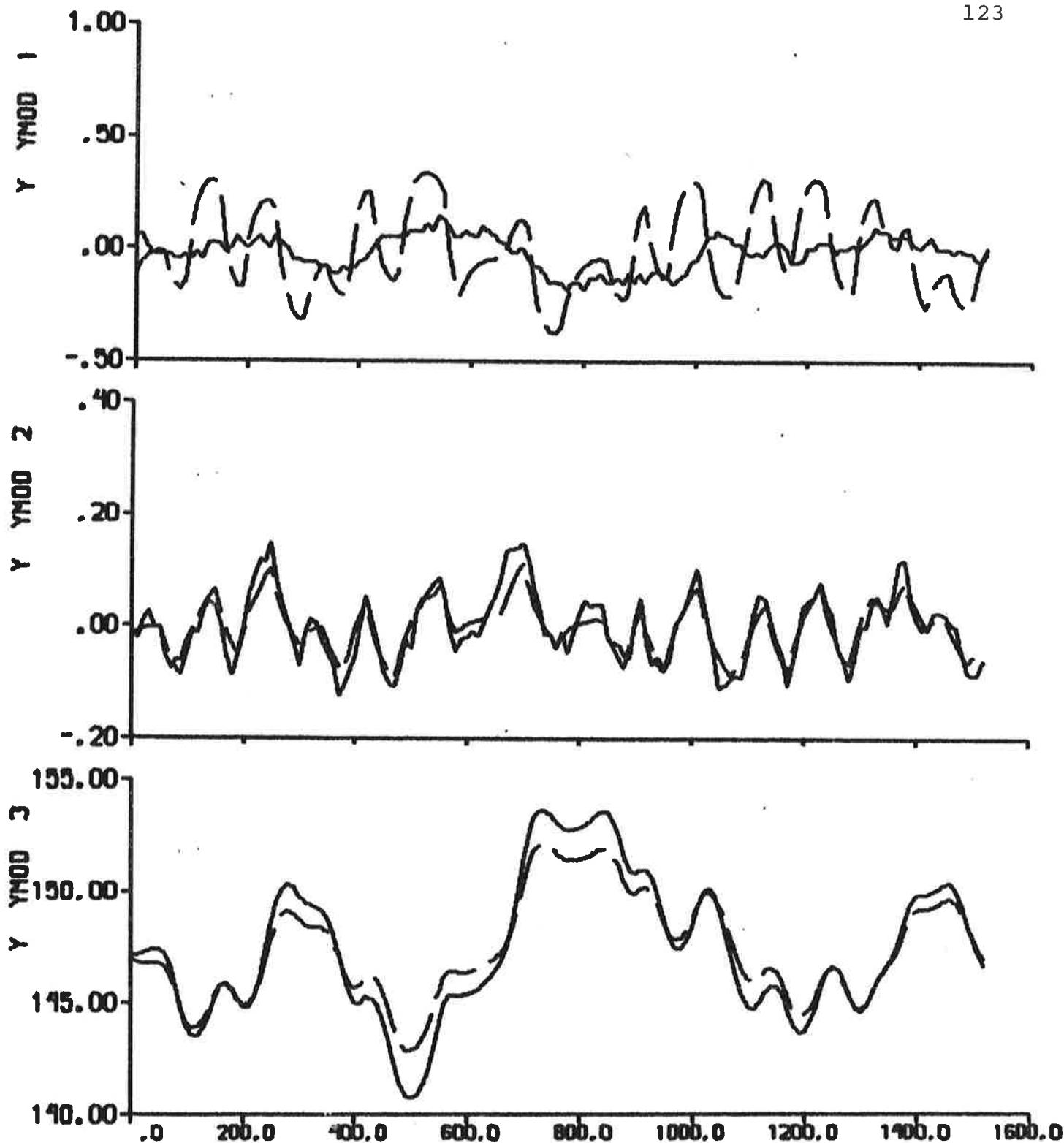
Fig. 5.10a - Result of output error identification to data from experiment E4, when the linear part of the model is fixed to SSPA:s model.
