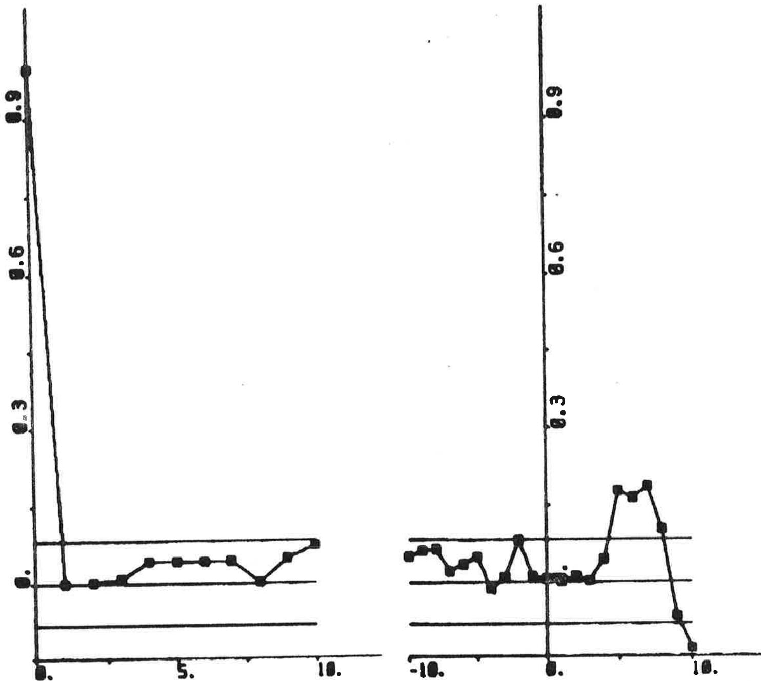
Fig. 6.53 - Autocorrelation function of residuals and cross correlation function between rudder input and residuals, where the residuals are obtained from ML identification using IDPAC to data from experiment E1 (3rd order model).
