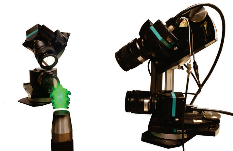
Figure 6.9 The camera arrangement used for measurements in vertically oriented volumes above the burner. The height of the measurement volume was ~50 mm. (Photo and editing A. & A. Petersson.)
