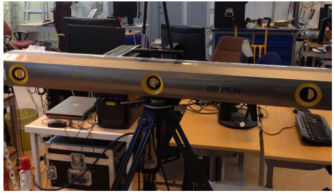
Figure 2.3 Experimental setup for milling experiments (left) at Lund University, including an optical tracking system (right) for high-accuracy measurements of robot position and orientation.
