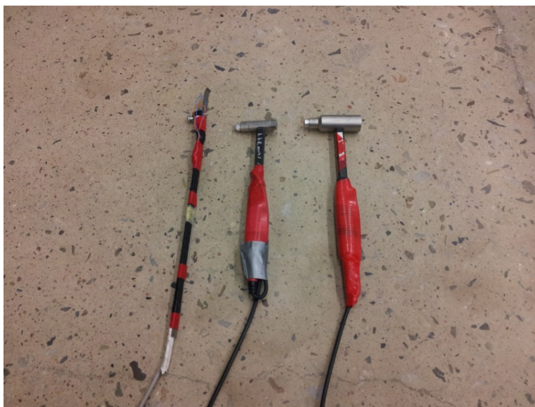
Figure 5.4: Impact hammers, from left: home-made impactor (screw/bolt) with piezoelectric crystal, hammer PCB model 086C03, hammer PCB model 086D05.
