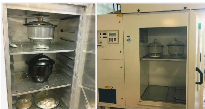
Figure 16. Storage set-up used in the present work. The samples were placed in open Petri dishes inside the desiccators at pre-set relative humidities, and then in the incubator to reach the desired temperature.
