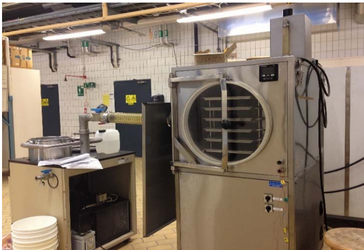
Figure 11. The freeze-dryer used (Labconco). The sample materials that had been frozen in metal containers were placed on the shelves inside the drying chamber.
