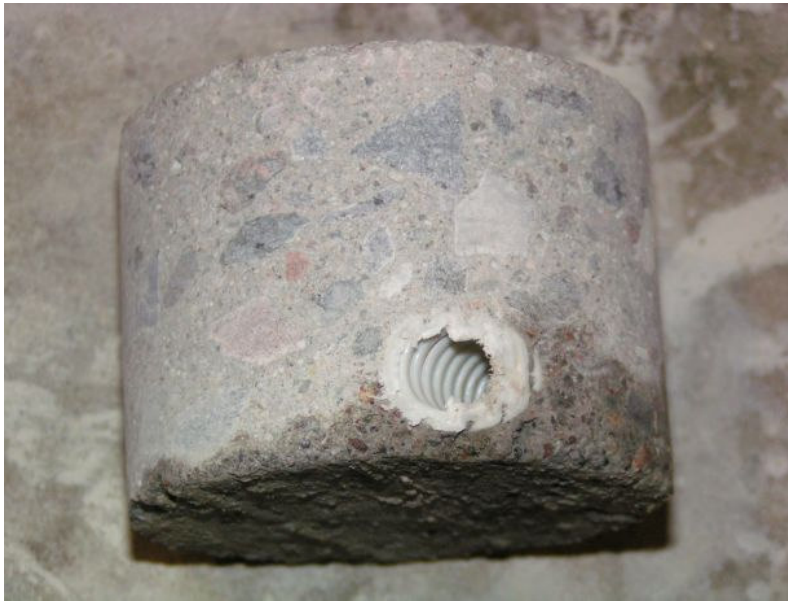
Figure 5.11 Fracture of cylinders when bond testing occurred totally within the interface between the HD/F element and the cast top layer. Note the proper filling beneath the installation tube though.
