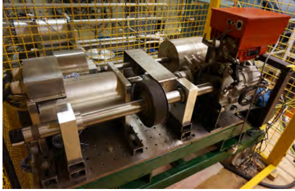
Figure A.3: The parallel drive bench with the iPMSM
