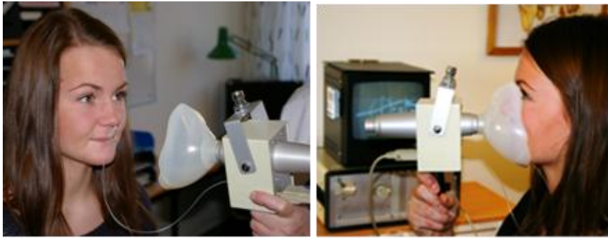
Figure 8. A transparent face mask, similar to that used for administering general anaesthesia is used, incorporating a pneumotachograph and connected to an amplifier and a recorder. “Patient”: Sara Thulesius.
