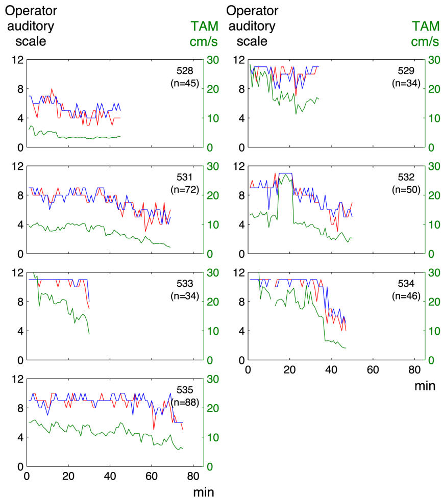
Figure 6. Operator auditory scale and time average mean velocity for individual Doppler recordings in the embolization model. Green line: time average mean velocity (TAM) (right y-axis); red line: sonographer's auditory perception; blue line: auditory perception supported by visual presentation of the spectrum (left y-axis); n: number of observations per lamb. doi:10.1371/journal.pone.0064033.g006
