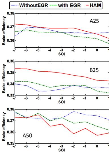
Figure 13. Brake efficiency vs. SOI. Top A25, Middle B25, Bottom A50
