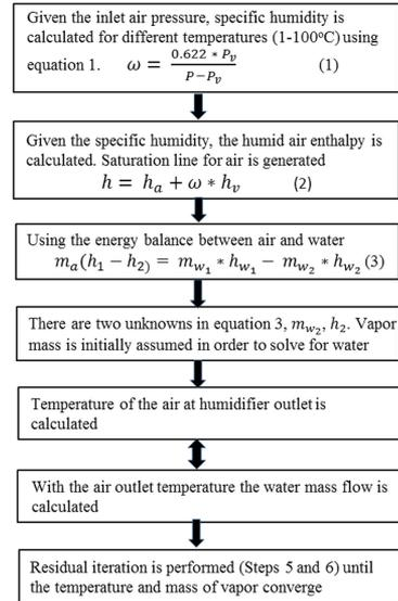
Figure 6. Humidification tower model working procedure
