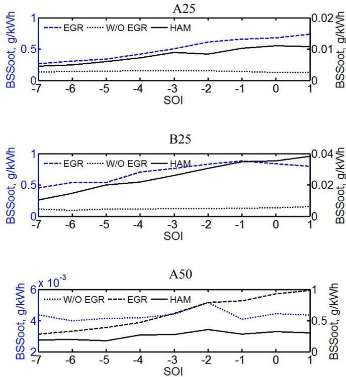
**Figure 28.** BSSoot vs. SOI. Top A25, Middle B25, Bottom A50
