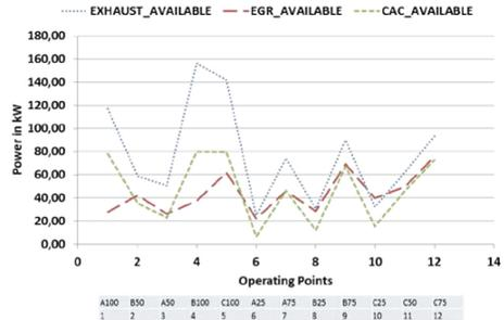
Figure 6. Energy availability in typical HD diesel engine.
