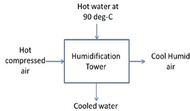
**Figure 2. Humidification tower simplified**
