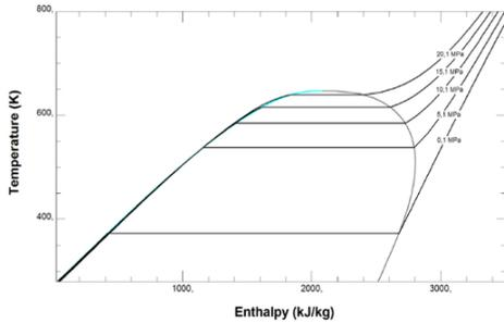
**Figure 7. T-h diagram of water at five different pressure levels**
