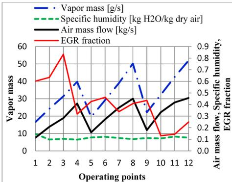
Figure 7. Inlet charge air at different operating points
