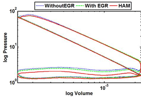
Figure 22. LogP-logV diagram (B25, SOI:+1)
