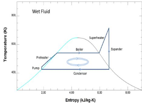
Figure 3. T-S diagram of water with typical Rankine cycle
