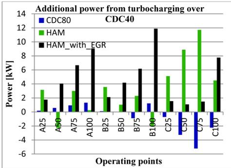
Figure 13. Potential turbine benefit with 80% constant efficiency
