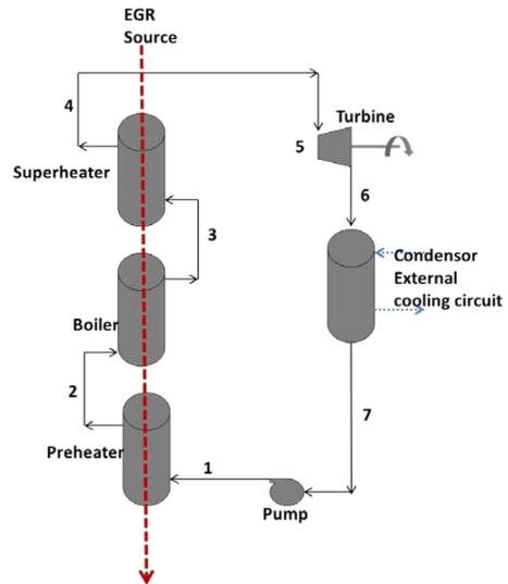
Figure 4. EGR as source: 1. Pressurized water; 2. Preheated water; 3. Boiled water vapor; 4. Super-heated steam; 5. Expander; 6. Steam after expansion; 7. Condensed water.
