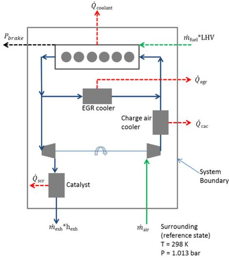
Figure 5. Energy flow (with system boundary)
