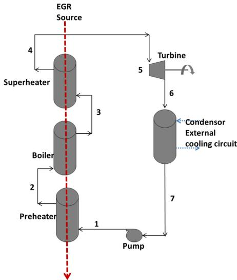
Figure 5. 1. Pressurized water; 2. Preheated water; 3. Boiled water vapor; 4. Superheated steam; 5. Expander; 6. Steam after expansion; 7. Condensed water.
