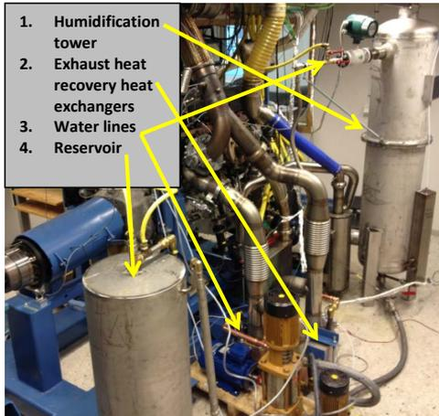
**Figure 6. Installation of components on HD engine**
