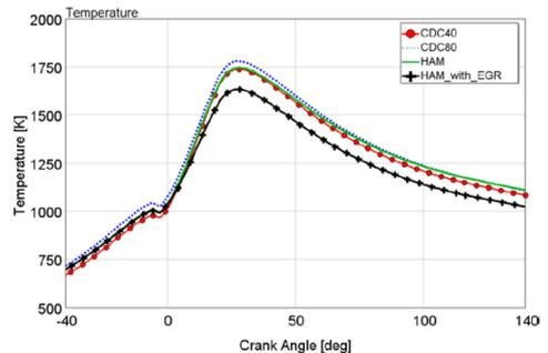
Figure 9. In-cylinder temperature
