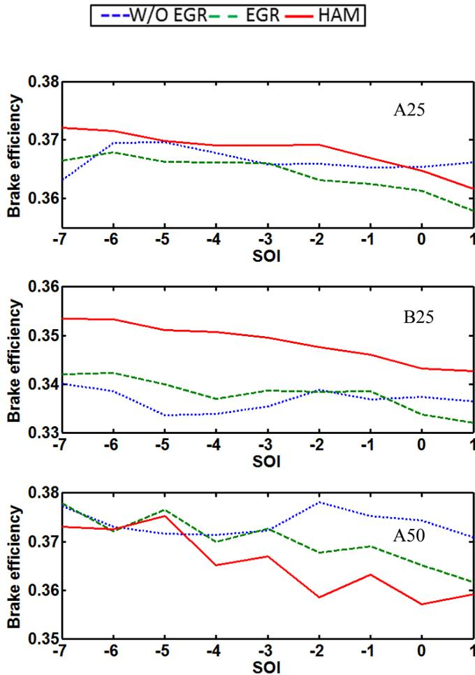
**Figure 29.** Brake efficiency vs. SOI. Top A25, Middle B25, Bottom A50
