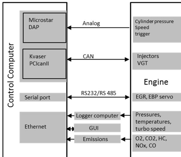
Figure 17. Engine communication
