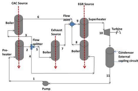
**Figure 8.** 1. Pressurized water; 2, 3, 4 & 5. Preheated water; 6, 7, 8 & 9. Boiled water vapor to superheater; 10. Superheated steam expansion; 11. Condensed water.
