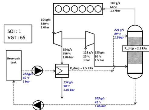
Figure 8. HAM layout with flows, temperatures, and pressures
