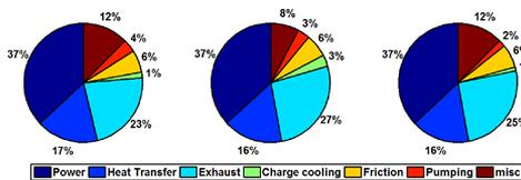
Figure 14. Energy Split for operating point A25 (Left: Without EGR, middle: With EGR, Right: HAM)
