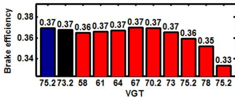
Figure 18. Brake efficiency vs. VGT at SOI: -6 (Blue: Without EGR, Black: With EGR, Red: HAM VGT sweep)
