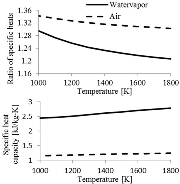
**Figure 3.** Specific heat capacities and ratios of specific heat capacities of air and water vapor
