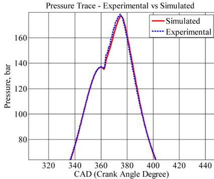
Figure 1. Pressure trace comparison between experimental and simulation
