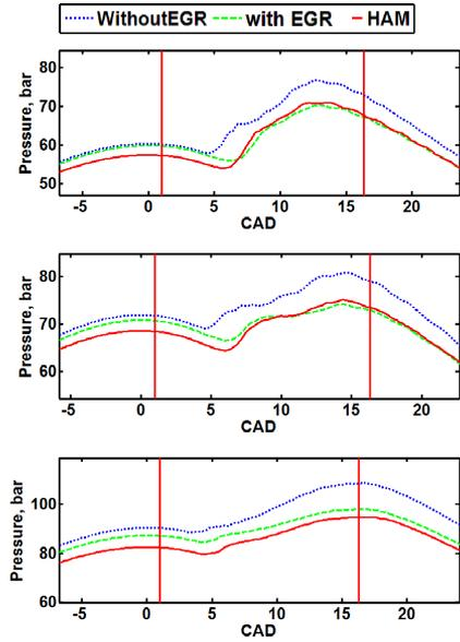
Figure 21. Cylinder Pressure vs CAD (at SOI: +1). Top: A25, Middle: B25, Bottom: A50
