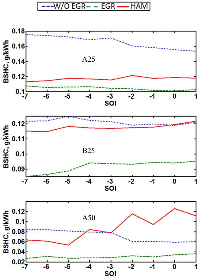
Figure 27. BSHC vs. SOI. Top A25, Middle B25, Bottom A50
