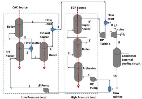
**Figure 9.** LP cycle (1. Pressurized water; 2, 3 & 4. Preheated water; 5, 6 & 7. Boiled water vapor to LP expander; 10. Condensed water); HP cycle (1'. Pressurized water; 2'. Preheated water; 3'. Boiled water vapor to superheater; 4'. Superheated steam expansion).
