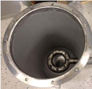
Figure 13. Humidification tower shell (upside down) with provisions for nozzles
