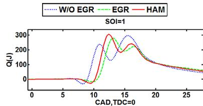
Figure 9. The rate of heat release
