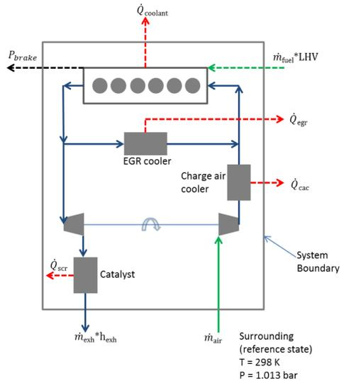
**Figure 2. Energy flow (with system boundary).**
