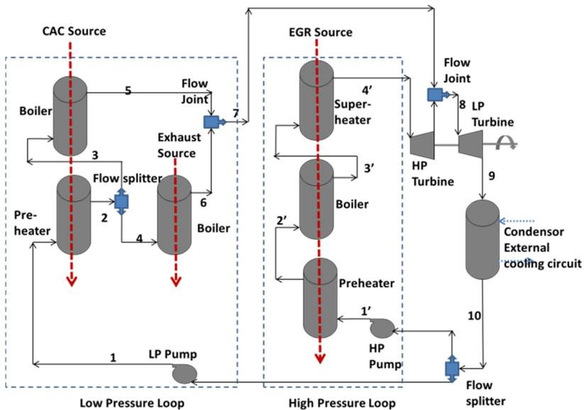
Figure 11. Dual loop Rankine cycle
