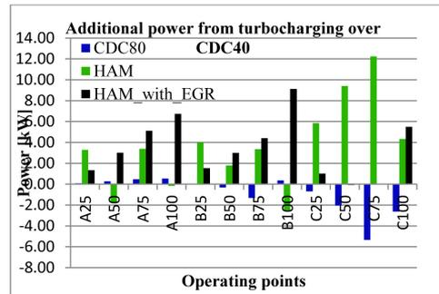
Figure 12. Potential turbine benefit with 75% constant efficiency
