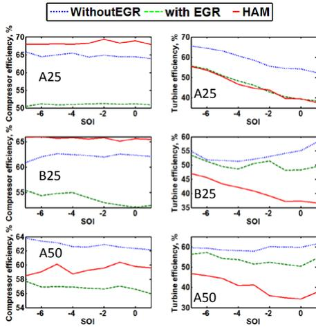
Figure 17. Turbine and compressor efficiency. Top A25, Middle B25, Bottom A50
