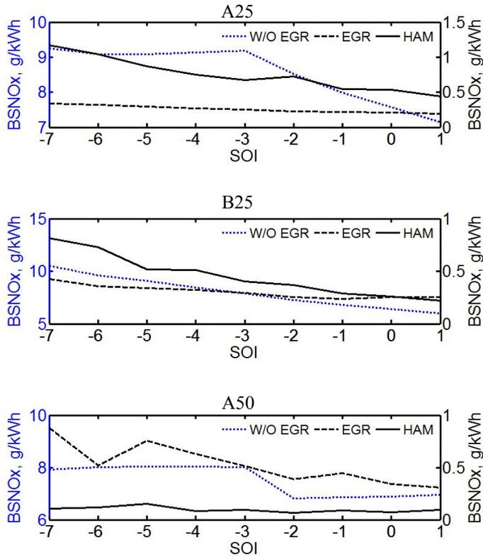
**Figure 25.** BSNOx vs. SOI. Top A25, Middle B25, Bottom A50
