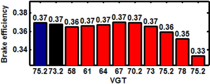
**Figure 34.** Brake efficiency vs. VGT at SOI: -6 (Blue: Without EGR, Black: With EGR, Red: HAM VGT sweep)
