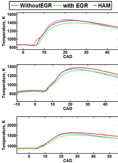
Figure 20. Cylinder temperature vs CAD (at SOI: +1). Top: A25, Middle: B25, Bottom: A
