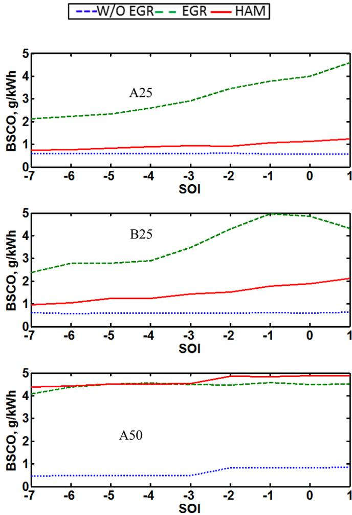
Figure 26. BSCO vs. SOI. Top A25, Middle B25, Bottom A50
