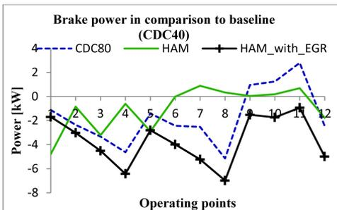
Figure 10. Brake power of different models in comparison with baseline (CDC40)
