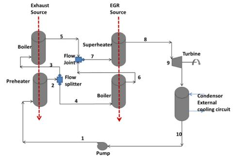
Figure 7. 1. Pressurized water; 2, 3 & 4. Preheated water; 5 & 6. Boiled water vapor; 7. Combined vapor to superheater; 8. Superheated steam; 9. Expander; 10. Steam after expansion and condensed water.
