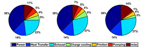
Figure 16. Energy Split for operating point A50 (Left: Without EGR, middle: With EGR, Right: HAM)
