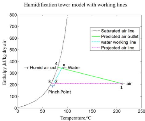
Figure 5. Humidification tower model with working lines
