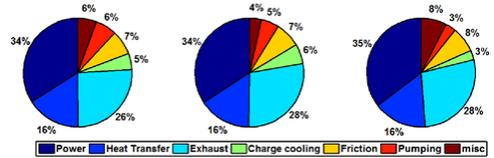
Figure 15. Energy Split for operating point B25 (Left: Without EGR, middle: With EGR, Right: HAM)
