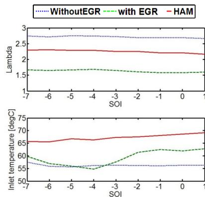
**Figure 7. Temperature and Lambda of three different modes (Operating point: B25)**
