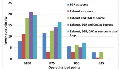
Figure 10. Comparison of different configuration of sources for Rankine cycle WHR for different operating load points
