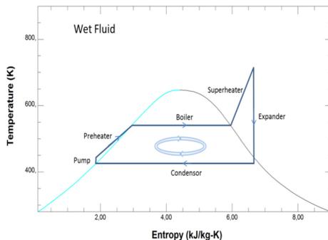
*Figure 1. T-S diagram of water with typical Rankine cycle.*
