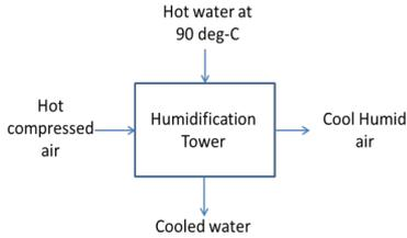
**Figure 2. Humidification tower; temperature overview**
