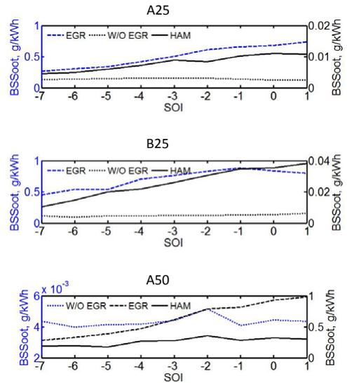
Figure 12. BSSoot vs. SOI. Top A25, Middle B25, Bottom A50
