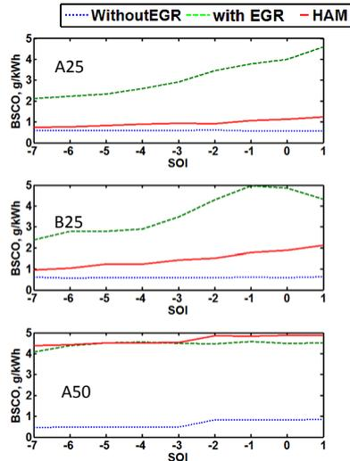
Figure 10. BSCO vs. SOI. Top A25, Middle B25, Bottom A50
