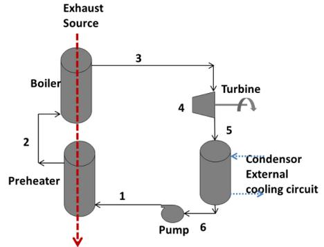
Figure 6. 1. Pressurized water; 2. Preheated water; 3. Boiled water vapor; 4. Expander; 5. Steam after expansion; 6. Condensed water.
