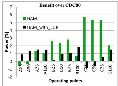
**Figure 4. The benefit of HAM over conventional diesel compared with similar Inlet temperature (80 °C).**
