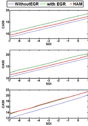
Figure 19. CA50 vs SOI. Top: A25, Middle: B25, Bottom: A50
