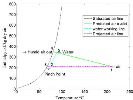
**Figure 3. h-T diagram of humidification process**
