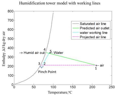
Figure 3. Enthalpy-Temperature diagram of humidification process
