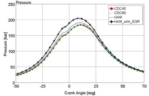
Figure 8. In-cylinder pressure
