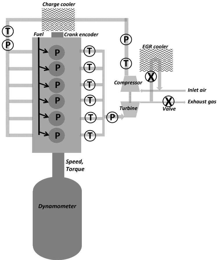
**Figure 16.** Engine Layout with valves, pressure, and temperature sensors.
