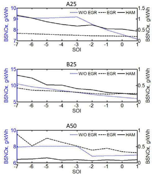
Figure 9. BSNOx vs. SOI. Top A25, Middle B25, Bottom A50
