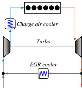
Figure 4. Conventional engine layout
