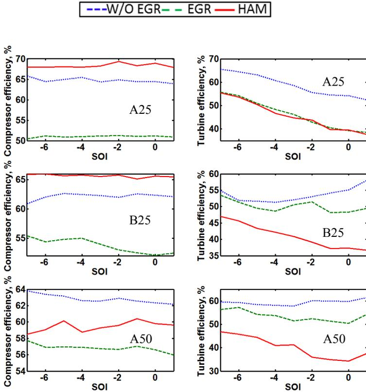
Figure 33. Turbine and compressor efficiency. Top A25, Middle B25, Bottom A50
