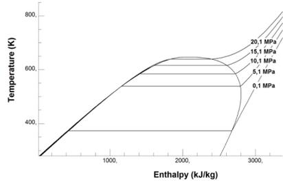
Figure 4. T-h diagram of water at five different pressure levels.
