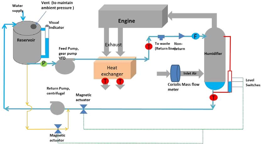
Figure 12. Graphical layout of the HAM system
