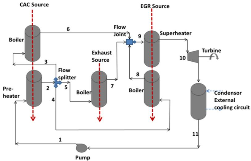
Figure 10. Single loop Rankine cycle with all three sources
