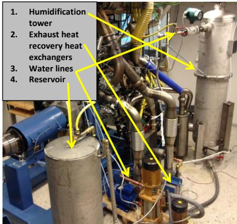
Figure 7. Installation of components on HD engine
