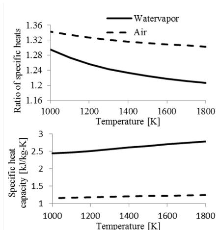
**Figure 1. Specific heat capacities and ratios of specific heat capacities of air and water vapor**
