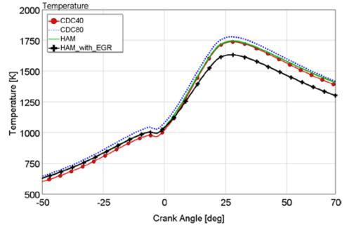
Figure 15. In-cylinder temperature
