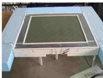
Fig. 4.2.5 The measuring area and the guarded ring.
