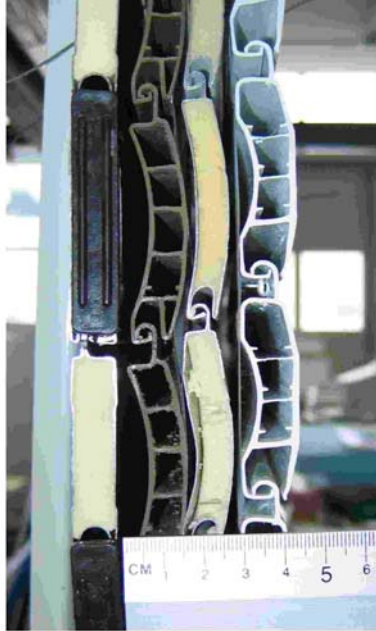
Fig. 4.2.7 Cross section of the profiles used in the shutters. From left to right: Shutter 2; Shutter 4; Shutter 1; Shutter 3.
