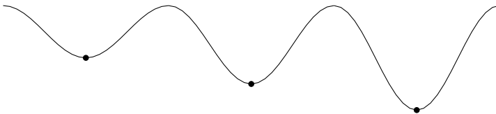
Figure 4.1 A nonconvex function with multiple minima. Depending on the starting point, a numerical optimization algorithm may end up in any of these.
