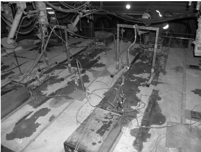
Fig. 1 Liquid water on the non-(fire)-exposed side of 200 mm thick concrete slabs.
