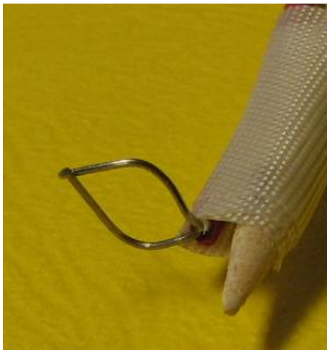
Figure 6 Welded thermocouple wire, diameter 0.5 mm.
