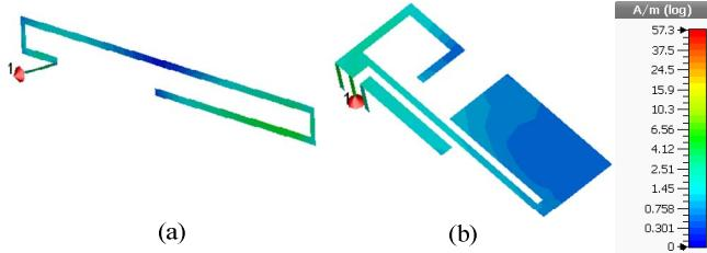
Fig. 8. Current distribution for monopole and PIFA antennas at 1.92 GHz.
