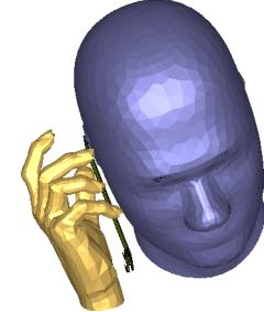
Fig. 6. Mobile handset with hand and head phantom.
