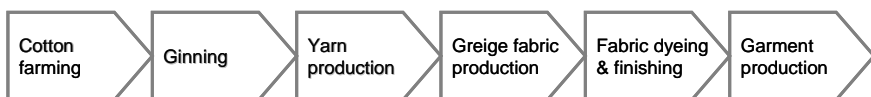
Figure 1-1: The product chain for a cotton garment showing only the production phase
