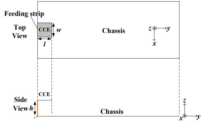
Fig. 1. Layout of the CCE on the 100 mm  $\times$  40 mm chassis.
