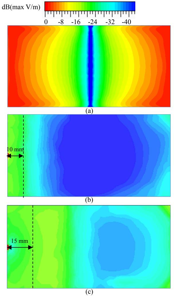
Fig. 6. Magnitude of electric near-field at 1.1 GHz on a 100 mm  $\times$  40 mm plane 3 mm above the chassis for (a) a standalone chassis (modal near-field), a chassis excited by the CCE with (b)  $l = 10$  mm and (c)  $l = 15$  mm.
