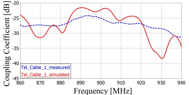
Fig. 10. Simulated and measured results for one of the cable routings for the receiving antenna above the rear seat (location 1).
