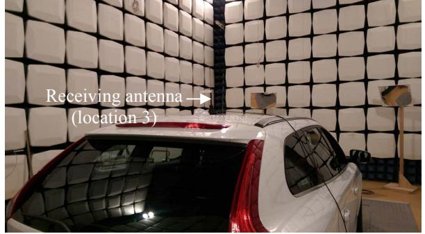
Fig. 3. Receiving antenna on the roof (receiving location 3).
