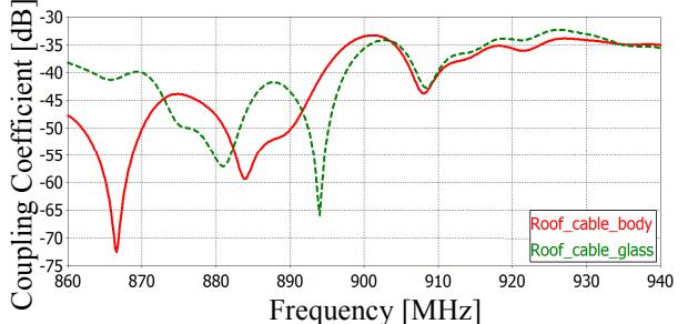
Fig. 11. Simulated channel with 2 different cable routings for the receiving antenna on the roof (location 3).
