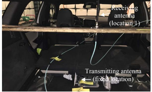
Fig. 1. Transmitting antenna below the rear seat and receiving antenna above the rear seat (receiving location 1).
