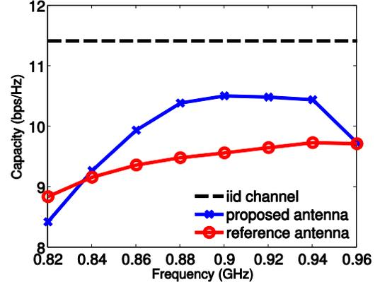
Fig. 11. Channel capacities for three different cases.
