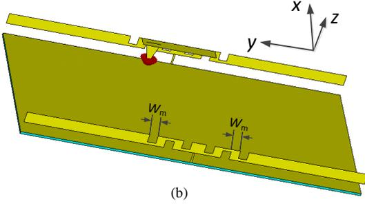
Fig. 6. Geometries of (a) T-strip antenna without meander line, and (b) T-strip antenna with meander line. The dimensions are:  $L_p = 30$  mm,  $W_p = 6$  mm,  $W_r = 2$  mm,  $W_m = 3$  mm. Other dimensions are identical to those in Fig. 2.
