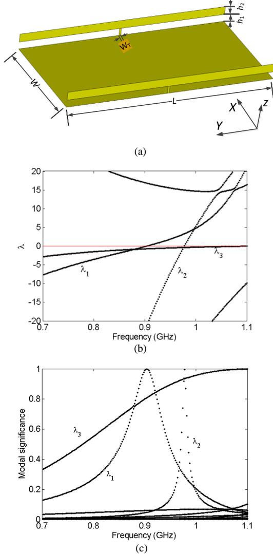
Fig. 2. (a) Geometries of the T-strip loaded chassis. The dimensions are:  $L = 120$  mm,  $W = 60$  mm,  $W_T = 0.5$  mm,  $h_1 = h_2 = 4$  mm. (b) Eigenvalues of the T-strip loaded chassis. (c) Modal significance of the T-strip loaded chassis.
