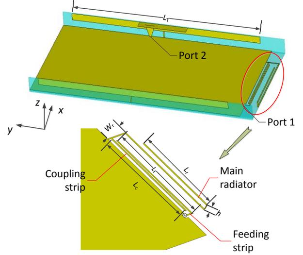
Fig. 8. Geometries of the proposed dual-antenna system. The dimensions are:  $L_T = 102$  mm,  $W_r = 4$  mm,  $L_c = 32$  mm,  $L_c = 37.5$  mm,  $L_t = 37.5$  mm,  $h = 3$  mm.
