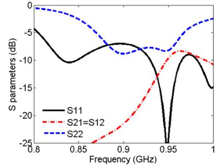
Fig. 9. S parameters of the proposed dual-antenna system.
