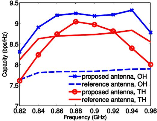
Fig. 15. Channel capacities for different user scenarios.
