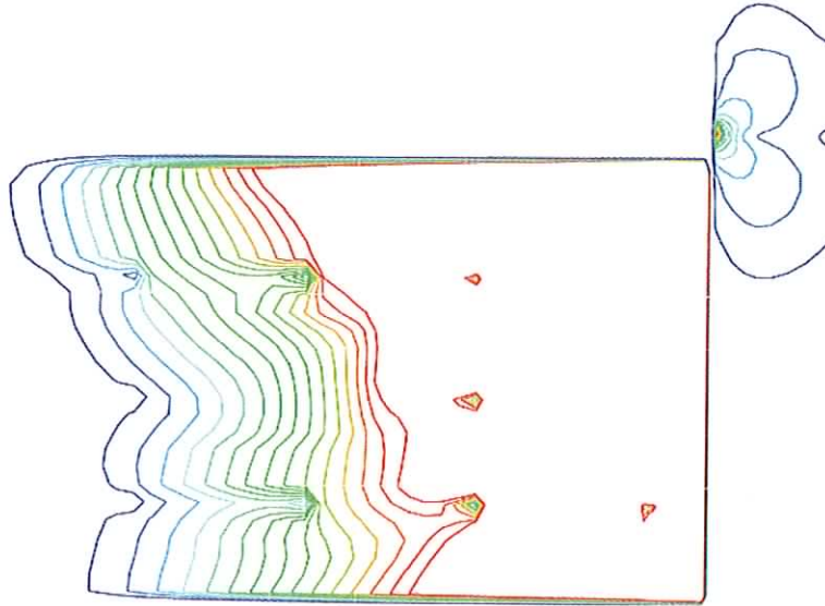
Figure 14 Horizontal view of temperature distribution in the fire room and in Marbella after 12 s for scenario #2. Plotting plane close to the ceiling in the Marbella room. The red line identifies the region where the temperature isotherm is 110 °C.
