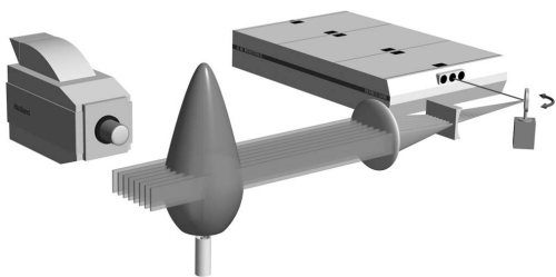
FIG. 6. Optical layout for three-dimensional imaging of formaldehyde.
