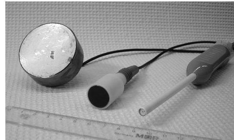
Figure 4. Three of the ultrasound transducers used in the experiments. From left: 50 mm diameter transducer with 100 mm geometrical focal length, 18 mm diameter plane transducer, and finally a 5 mm diameter ultrasound probe with a focal length of 1.5 mm and a central hole for water cooling.
