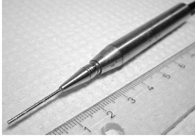
Figure 6. The needle hydrophone used for acoustic pressure measurements. The active tip of the hydrophone is 0.5 mm in diameter and the scale in the picture is in cm.
