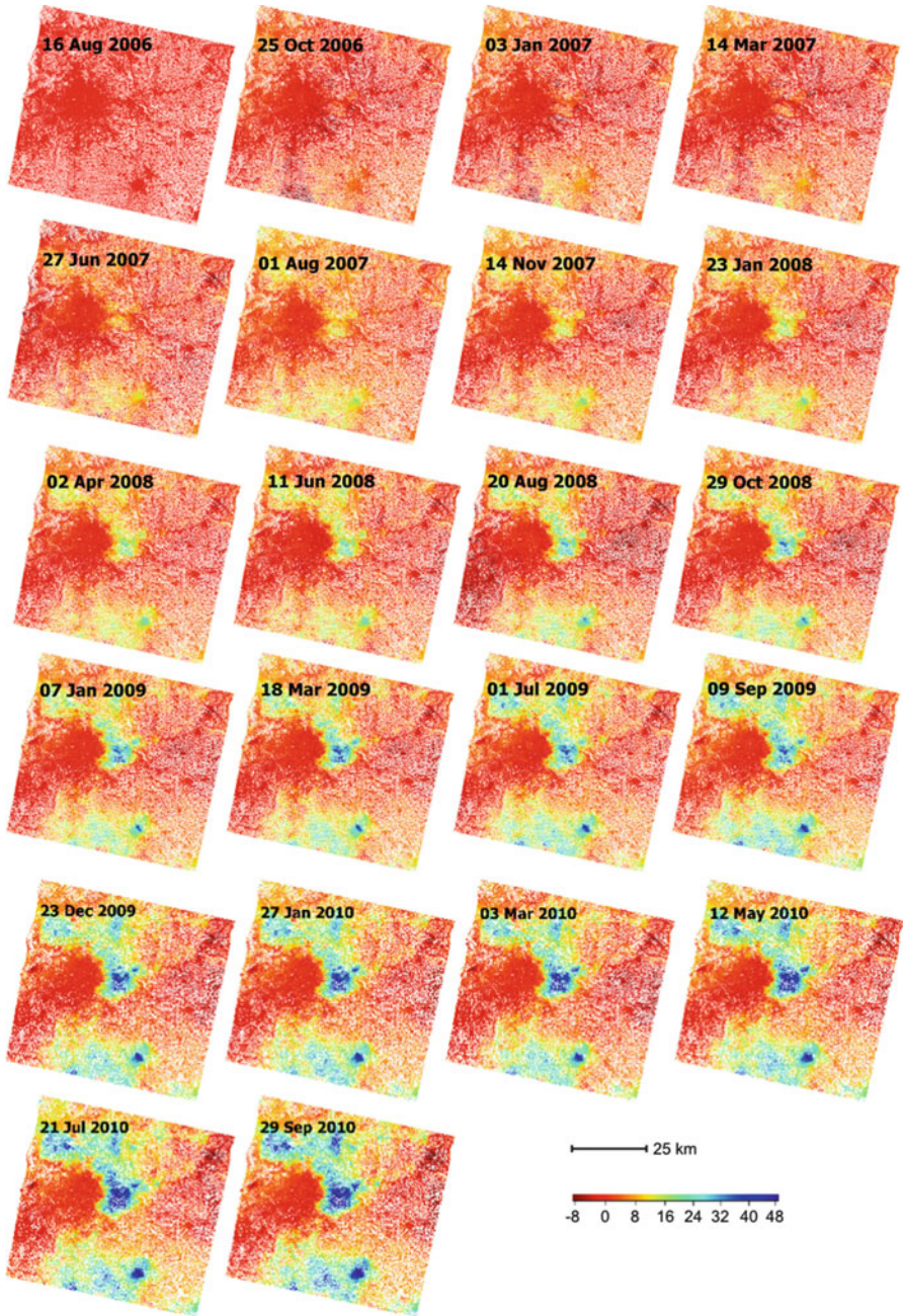
Fig. 19.8 Time series displacement (rad) in the direction of the PS point line of sight in the study area from 2006–2010
