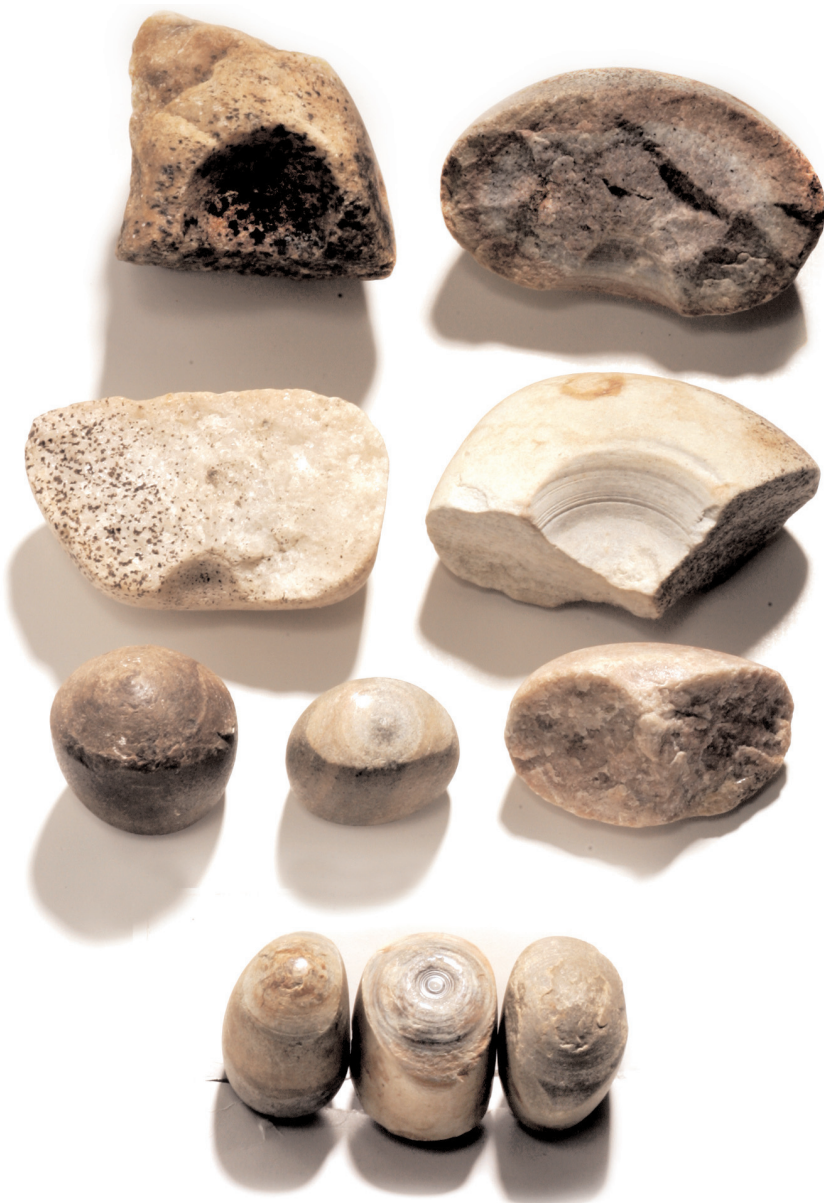
Fig. 3. Stone artefacts used during earlier times in the rotating machinery of the mill. All were collected under the water flowing only a few meters from the mill. First and second upper rows: four parts of circular stones belonging to the driving machinery. Third row: two small ovoid stones (highly polished) and a piece of a circular stone. Fourth row: three other small egg shaped stones which are also highly polished, some of them on both sides.
