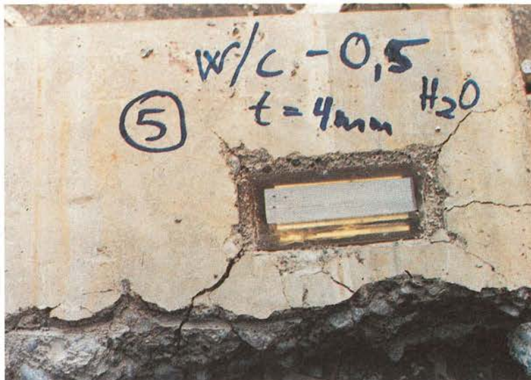
Photo 14. Corrosion cell in Series 1, cell No. 1 after conclusion of exposure.
