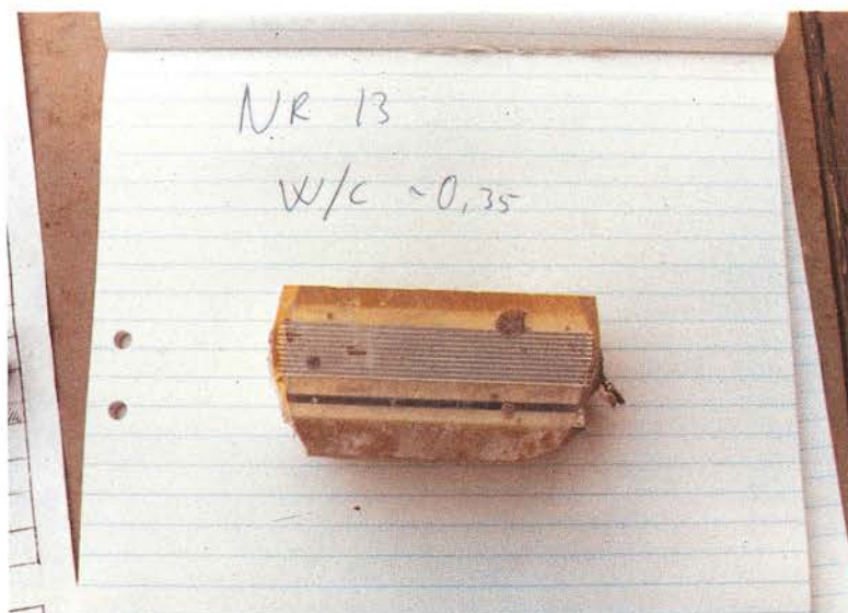
Photo 29. Corrosion cell where about 20% of the anodic area has begun to corrode. Note that the three steel plates show no more than local corrosion. Cell No. 13, in Series 2.
