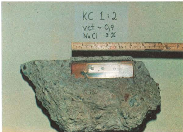
Photo 9. Embedded corrosion cell after concrete had been chipped away.
