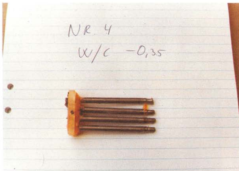
Photo 25. Unattacked corrosion cell. A varying oxide formation can, however, be seen along the cylindrical surfaces. When compared with the preceding photo, the differences are insignificant. Cell No. 4, in Series 2.
