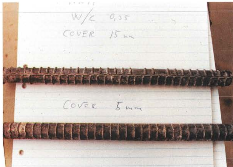
Photo 30. State of reference bars after exposure in series in Series 2. A certain discolouration can be noted along the cylindrical surface of all bars and all bars show limited pitting for a maximum of 1% of the total area.
