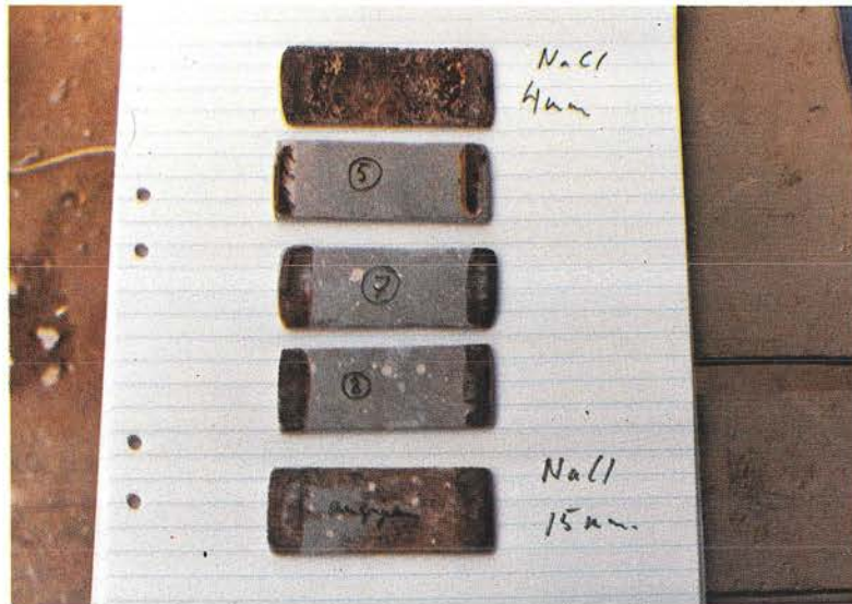
Photo 23. Steel plates contained in the same specimens as corrosion cells in Series 1. Counted from the top, the plates were contained in the following specimens:
