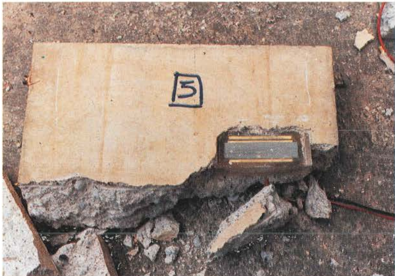
Photo 16. Corrosion cell in Series 1, cell No. 3 after conclusion of exposure.
