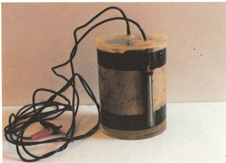
Photo 40. The process of corrosion stopped by repassivation or lack of O_2 . Cathode cast into concrete, anode in waterfilled space. Exposure time 5 years.
