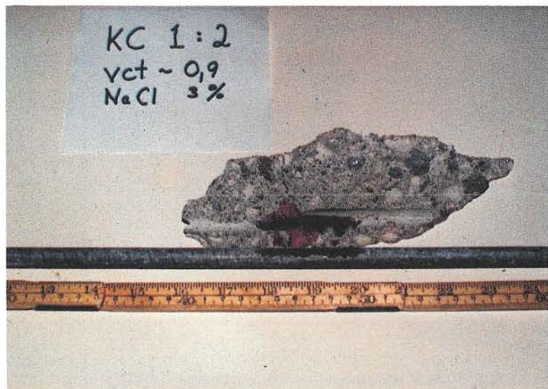
Photo 12. The reinforcement bars (the reference bars) also showed signs of corrosion attacks where the corrosion cells had indicated this.
