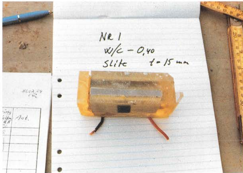
Photo 37. Cell No. 8 in Series 4. Slite Portland cement.
