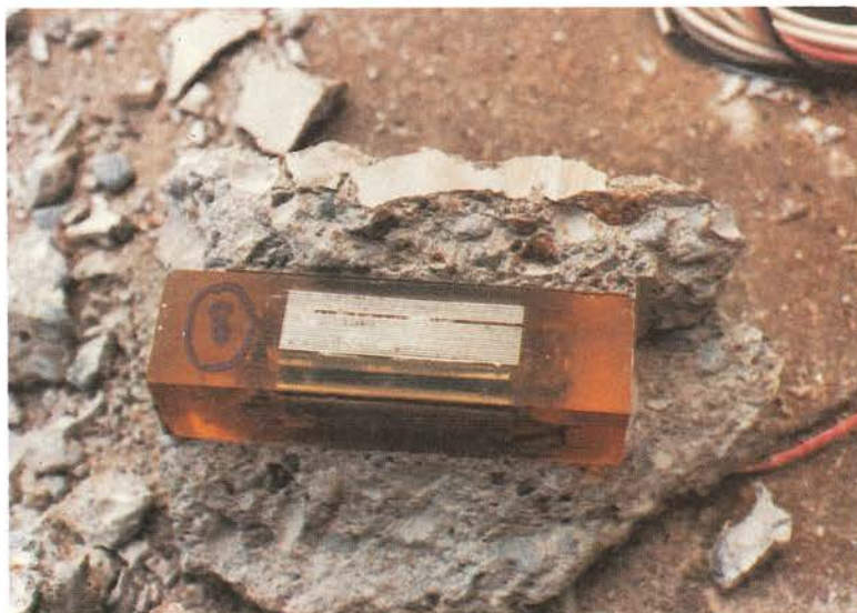
Photo 21. Corrosion cell in Series 1, cell No. 9 after conclusion of exposure.
