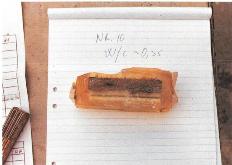
Photo 26. The entire corrosion cell has been attacked. Maximum pitting depth approximately 0.5 mm. Cell No. 10, in Series 2.
