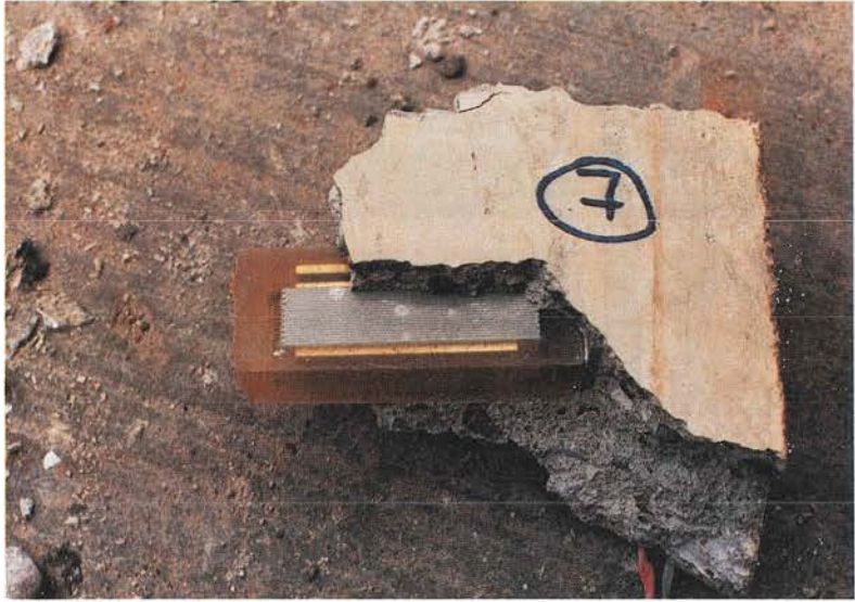
Photo 15. Corrosion cell in Series 1, cell No. 2 after conclusion of exposure.
