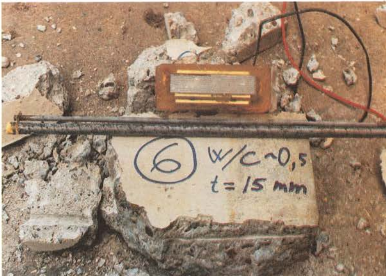
Photo 18. Corrosion cell in Series 1, cell No. 6 after conclusion of exposure.
